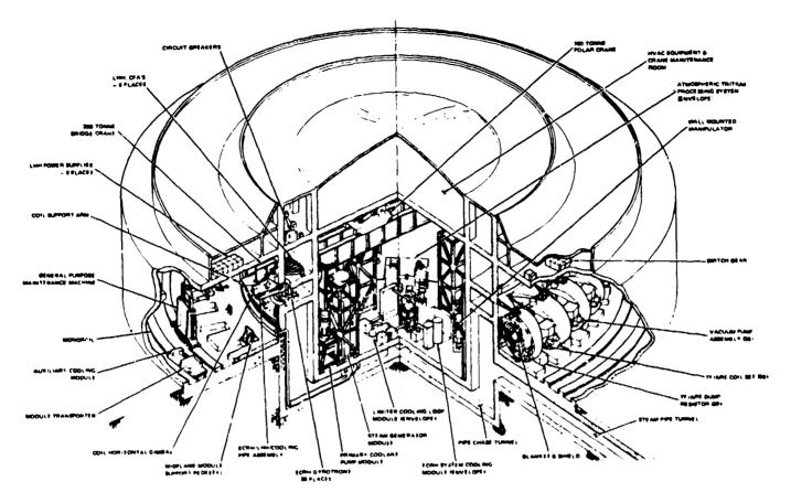
Fig. 1. EBT Reactor Building showing the interrelation of key reactor components.
