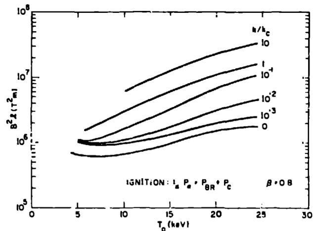
FIGURE 5. Dependence of  $B^2$ (ignition) on axial center temperature for a LMF device with material endplugs, including the constraint of classical alpha-particle thermalization.<sup>(28)</sup>
