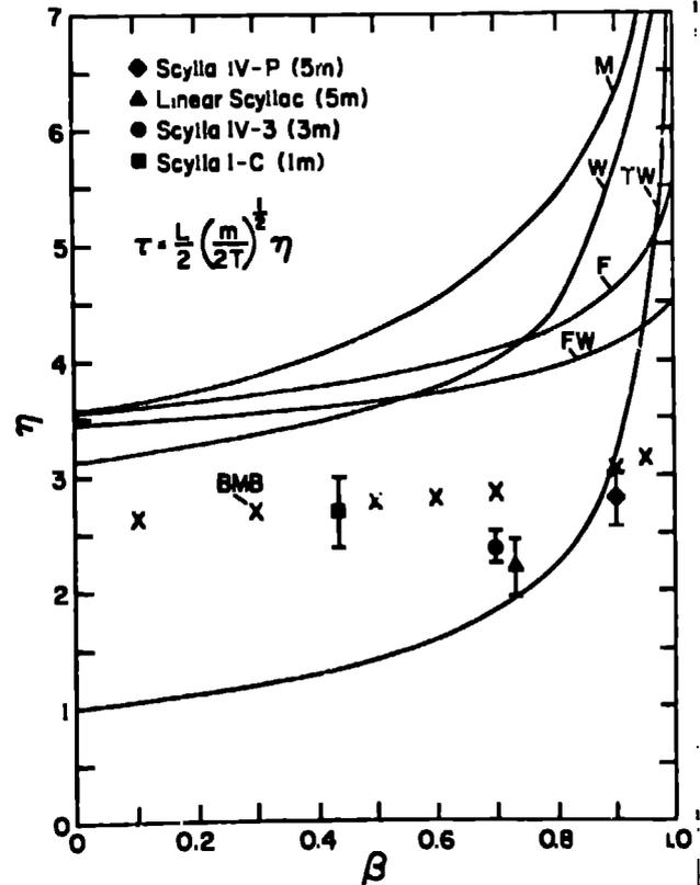
FIGURE 1. A comparison of theory and experiment for free streaming endloss from a LMF device (21): M(Ref. 22), W(Ref. 23), TW(Ref. 24), F(Ref. 25), FW(Ref. 19), BMB(Ref. 20).
