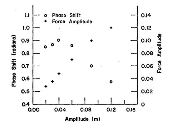
Fig. 1. Phase shift and amplitude of the dynamic pressure force as functions of the wedge displacement amplitude.
