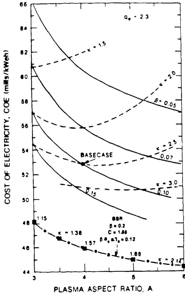
Fig. 2. Dependence of COE on plasma aspect ratio, A, and beta, B, for  $q_0 = 2.3$  with Eq. (20) enforced. Lines of constant plasma elongation,  $\kappa$ , are also shown. The  $\beta = 0.2$  SSR tokamak case is also included.
