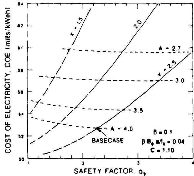
Fig. 3. Dependence of COE on  $q_0$  for a range of  $\kappa$  and A values that satisfy Eq. (20) with  $\beta = 0.1$  the basecase tokamak shown.
