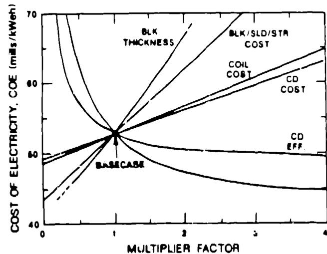
Fig. 4. Sensitivity of COE for the basecase tokamak on stability limits,  $\beta B_0 a / I_p$ , current-drive efficiency,  $I_p / P_{CD}$ , current-drive power costs, coil units costs, blanket shield/structural unit costs, and blanket thickness.
