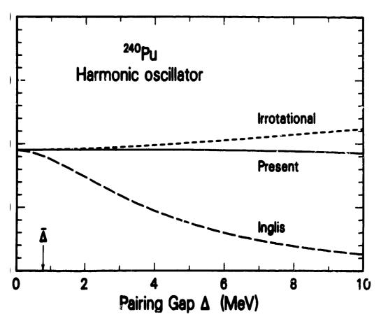
1. Dependence of the  $\beta$ -vibrational inertia upon the pairing gap  $\Delta$  in a harmonic-oscillator potential at the equilibrium deformation. The solid curve gives the present result calculated in the gencranking model with 15 oscillator shalls, the long-dashed curve corresponding result calculated in the Inglis cranking model and -dashed curve gives the irrotational result.
