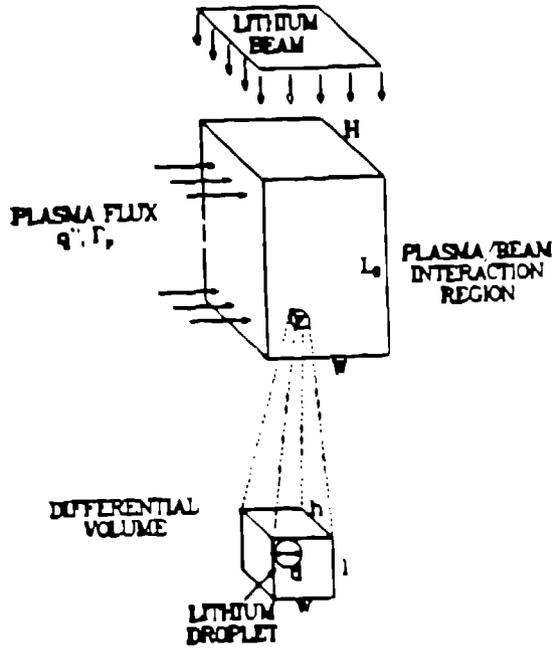
Fig. 4. Model of the LDB-plasma interaction zone and a differential volume element containing a single droplet
