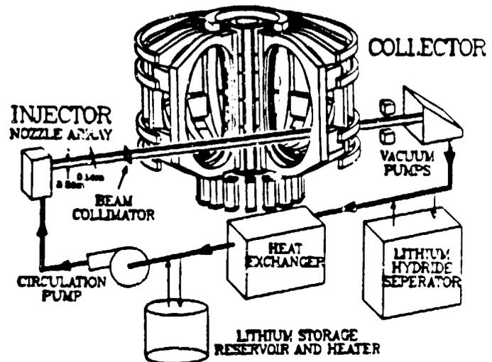
Fig. 1. Schematic of the LDB heat and particle collector drawn onto a view of the magnetic system assembly for ITER.<sup>1</sup>
