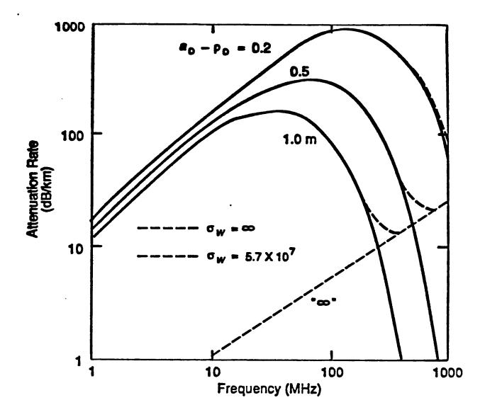
Attenuation rate of mode that behaves as axial surface wave at high frequencies for dielectric-coated conductor located in circular tunnel. Case indicated by " $\infty$ " corresponds to having conductor located in free space. For example shown, a=1mm, c=5mm, a=2m, a=2
