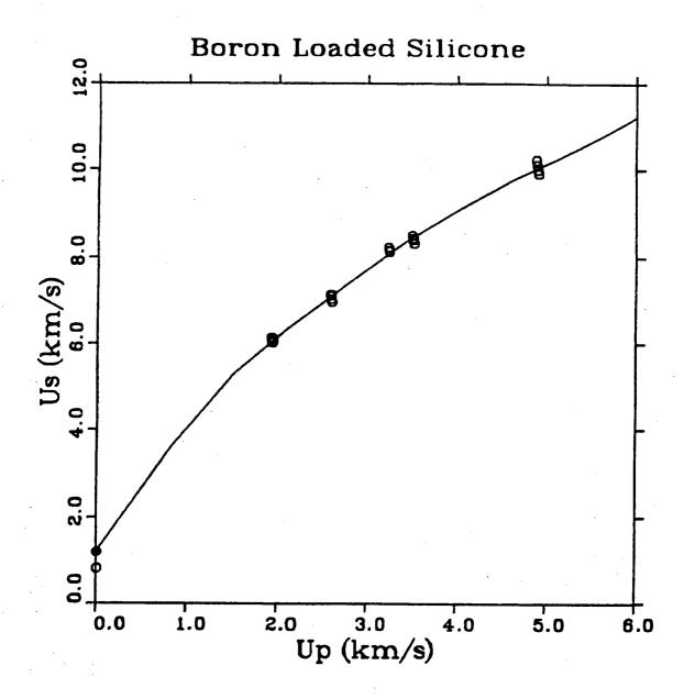
Figure 2. The theoretical Hugoniot for B-Silicone is compared with Hugoniot data and two experimental sound speeds. (Open circles are from Ref. 2, and the solid circle is from Ref. 9.)
