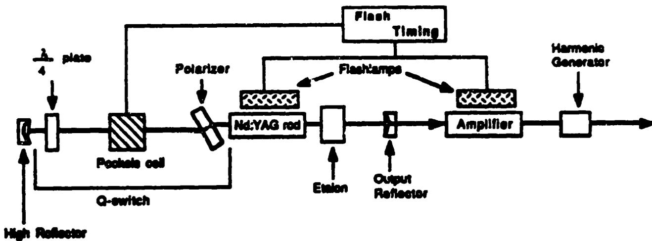
Figure 4.1: Schematic diagram of the Nd:YAG laser.
