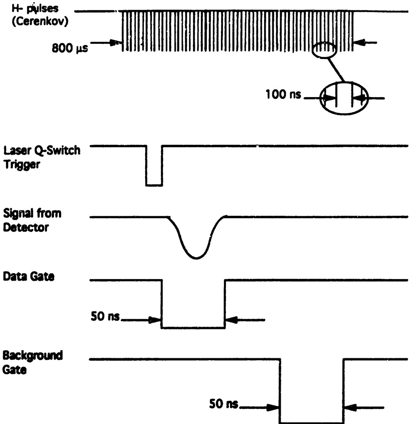
**Figure 5.7: Laser event and background timing diagram.**
