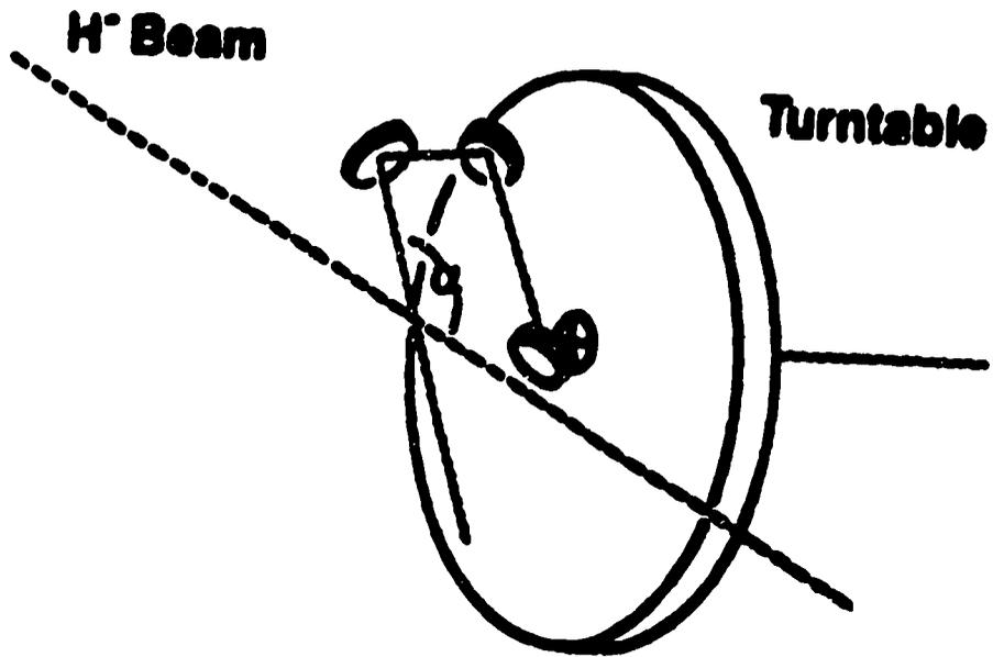
**Figure 3.6: The mirror arrangement or "spider".**
