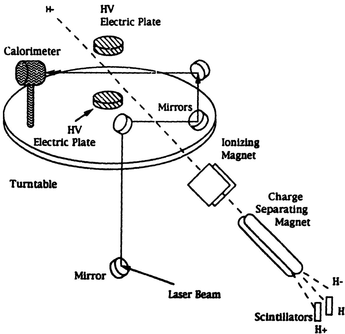
**Figure 3.7: The 1989 setup for electric field studies. Electric field plates were retracted for the zero-field work.**
