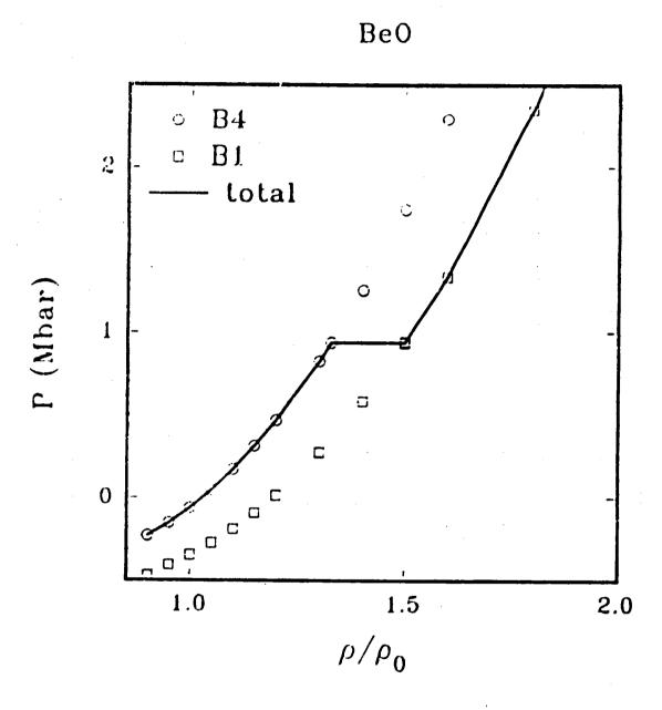
Figure 1 - The pressure vs. density points calculated via the FLMTO method for the B4 and B1 phases of BeO. The solid line is the 0 K isotherm which minimizes the Gibbs free energy.
