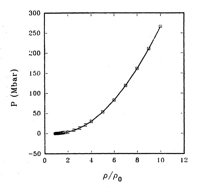
Figure 2 - Calculated 0 K isotherm for BeO obtained with FLMTO calculations.
