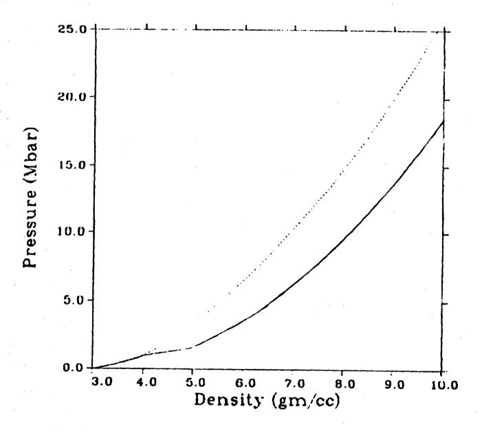
Figure 4 - Cold curves are shown for material numbers 7612 (solid line) and 7611 (dashed line).
