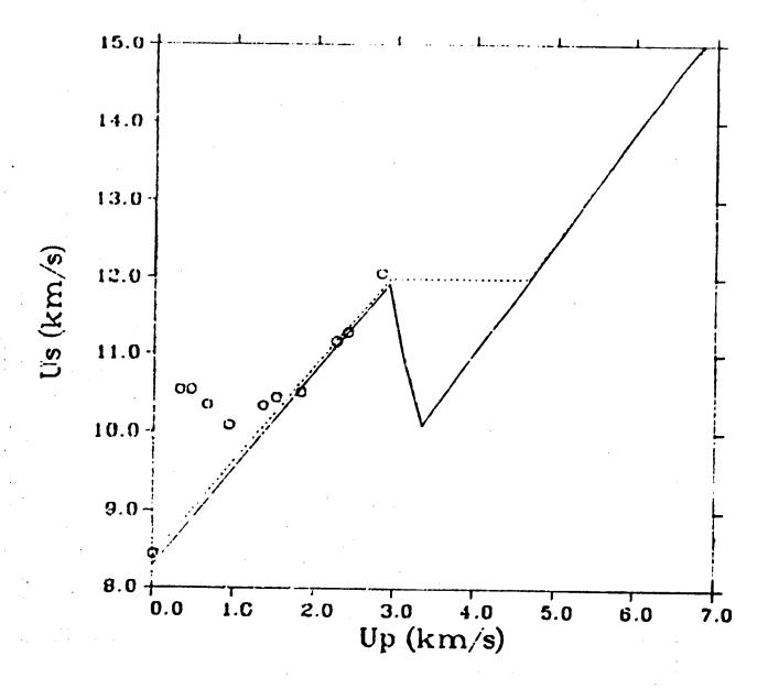
Figure 3 - The calculated principal Hugoniot for BeO (solid line) is compared to the experimental data of Ref. 6. Also shown is the straightline fit used in generating material number 7612 (dashed line).
