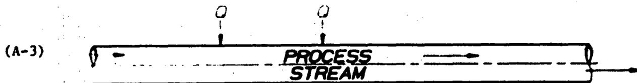
Figs. A-1, A-2, A-3: Three possible reactor configurations: (A-1) one-stream regenerative, (A-2) two-stream counterflow, and (A-3) one-stream single-pass.
