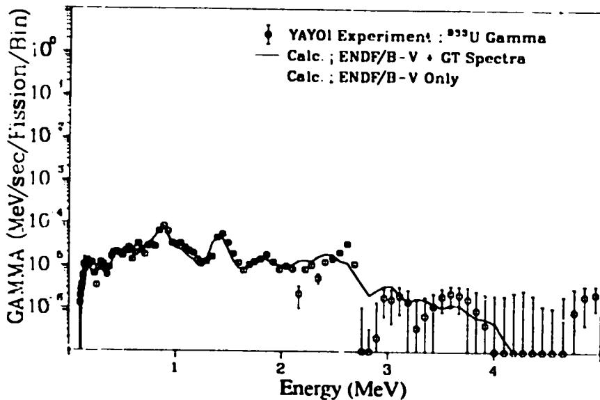
Fig. 182. Gamma spectrum after  $^{233}\text{U}$  fast neutron fission
