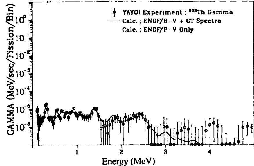
Fig. 375. Gamma spectrum after  $^{232}\text{Th}$  fast neutron fission
