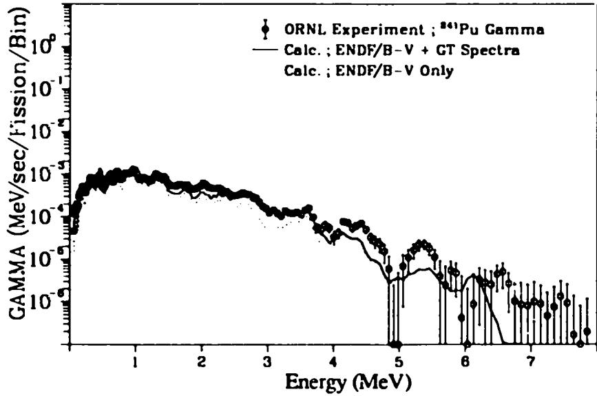
Fig. 130. Gamma spectrum after  $^{241}\text{Pu}$  thermal fission
