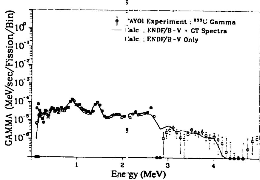
Fig. 179. Gamma spectrum after  $^{233}\text{U}$  fast neutron fission
