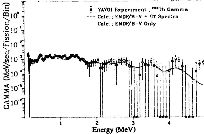
Fig. 338. Gamma spectrum after  $^{232}\text{Th}$  fast neutron fission
