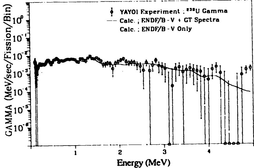
Fig. 243. Gamma spectrum after <sup>238</sup>U fast neutron fission
