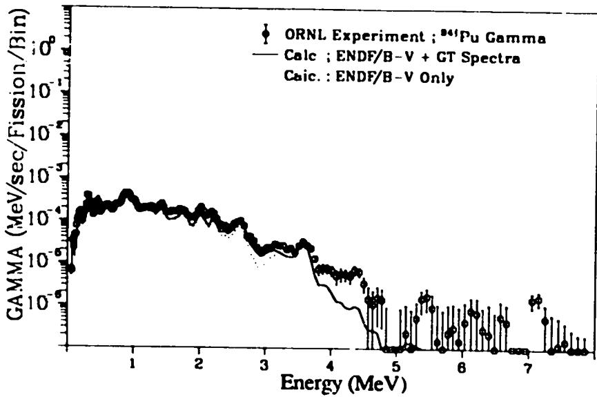
Fig. 134. Gamma spectrum after  $^{241}\text{Pu}$  thermal fission
