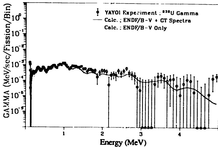
Fig. 251. Gamma spectrum after  $^{238}\text{U}$  fast neutron fission
