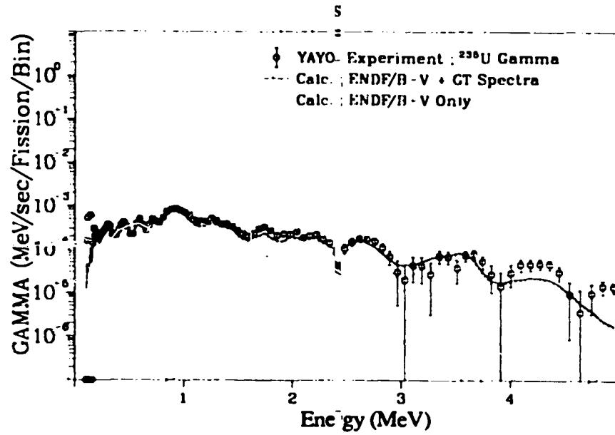
Fig. 219. Gamma spectrum after  $^{235}\text{U}$  fast neutron fission
