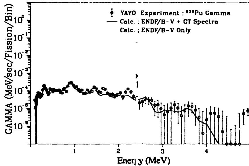
Fig. 306. Gamma spectrum after  $^{239}\text{Pu}$  fast neutron fission ( $T_{\text{irrad.}} = 10.0$  sec,  $T_{\text{cool.}} = 2000.0$  sec).
