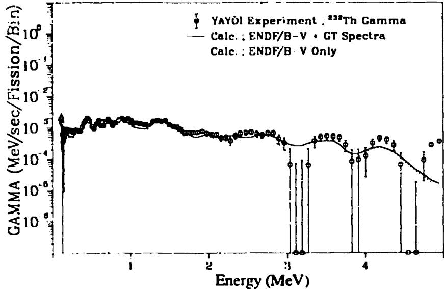
Fig. 352. Gamma spectrum after  $^{232}\text{Th}$  fast neutron fission ( $T_{\text{irrad.}} = 100.0$  sec,  $T_{\text{cool.}} = 230.0$  sec).
