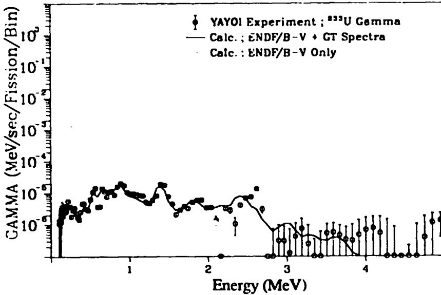
Fig. 186. Gamma spectrum after  $^{233}\text{U}$  fast neutron fission
