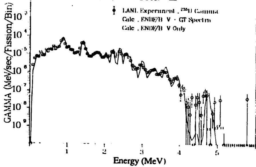
Fig. 393. Gamma spectrum after  $^{235}\text{U}$  thermal neutron fission
