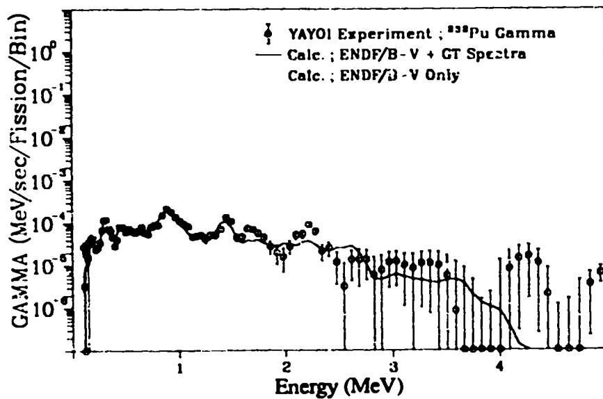
Fig. 308. Gamma spectrum after  $^{239}\text{Pu}$  fast neutron fission
