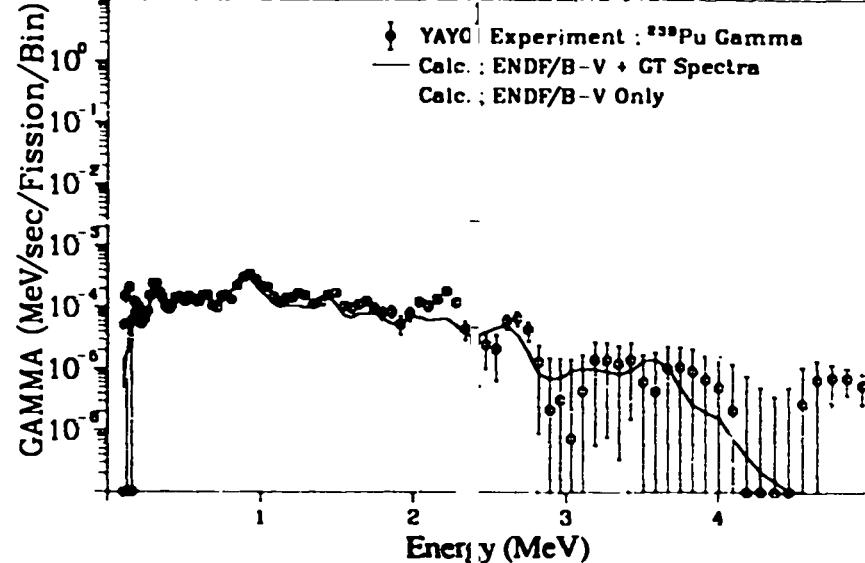
Fig. 305. Gamma spectrum after  $^{239}\text{Pu}$  fast neutron fission ( $T_{\text{irrad.}} = 10.0$  sec,  $T_{\text{cool.}} = 1600.0$  sec).
