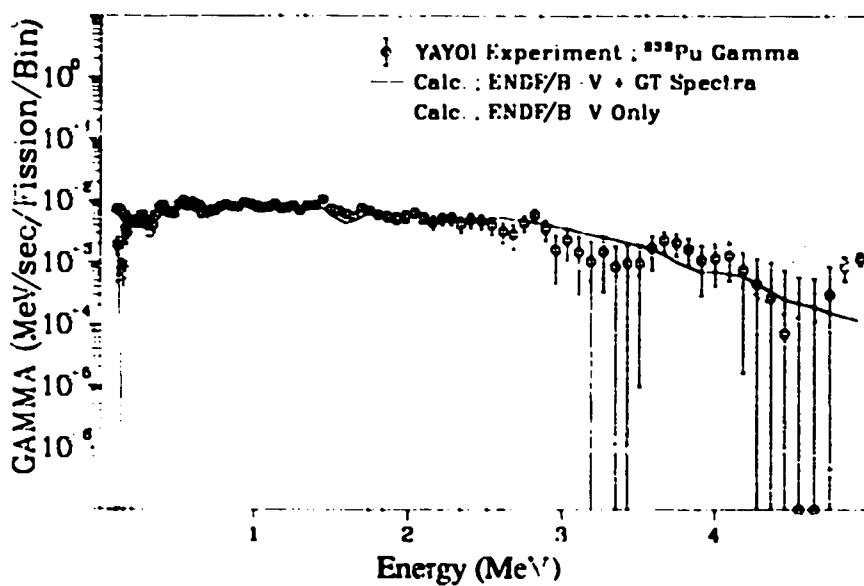
Fig. 288. Gamma spectrum after  $^{239}\text{Pu}$  fast neutron fission ( $T_{\text{irrad.}} = 10.0 \text{ sec.}$ ,  $T_{\text{cool.}} = 26.0 \text{ sec.}$ ).
