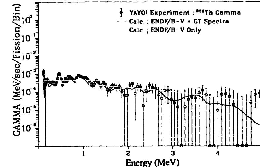
Fig. 343. Gamma spectrum after  $^{232}\text{Th}$  fast neutron fission ( $T_{\text{irrad.}} = 10.0$  sec,  $T_{\text{cool.}} = 700.0$  sec).
