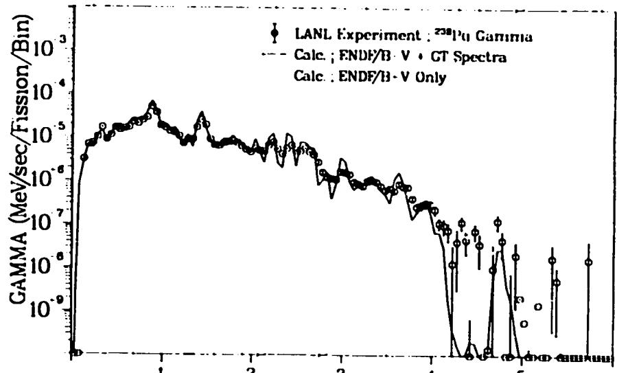
Fig. 405. Gamma spectrum after  $^{239}\text{Pu}$  thermal neutron fission
