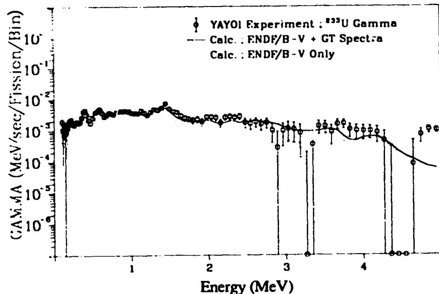
Fig. 194. Gamma spectrum after  $^{235}\text{U}$  fast neutron fission
