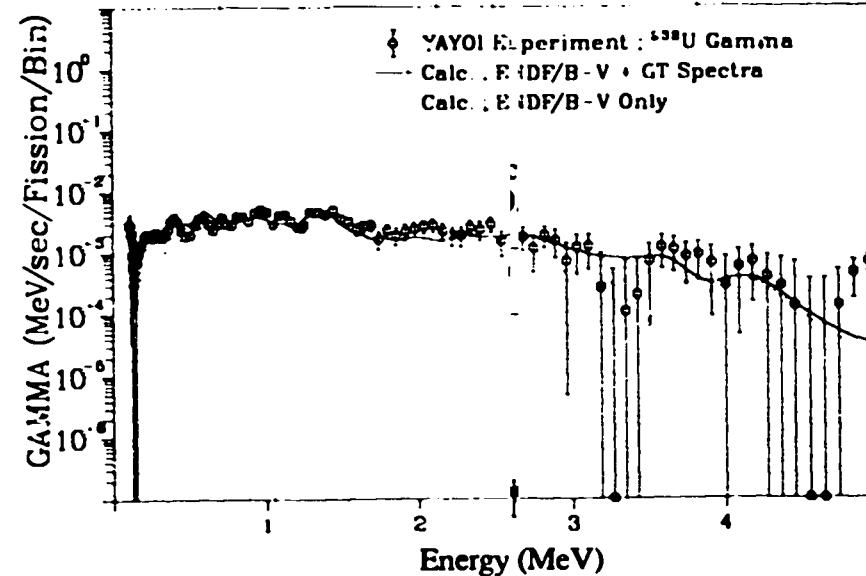
Fig. 245. Gamma spectrum after <sup>238</sup>U fast neutron fission
