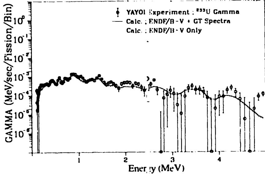
Fig. 156. Gamma spectrum after  $^{233}\text{U}$  fast neutron fission
