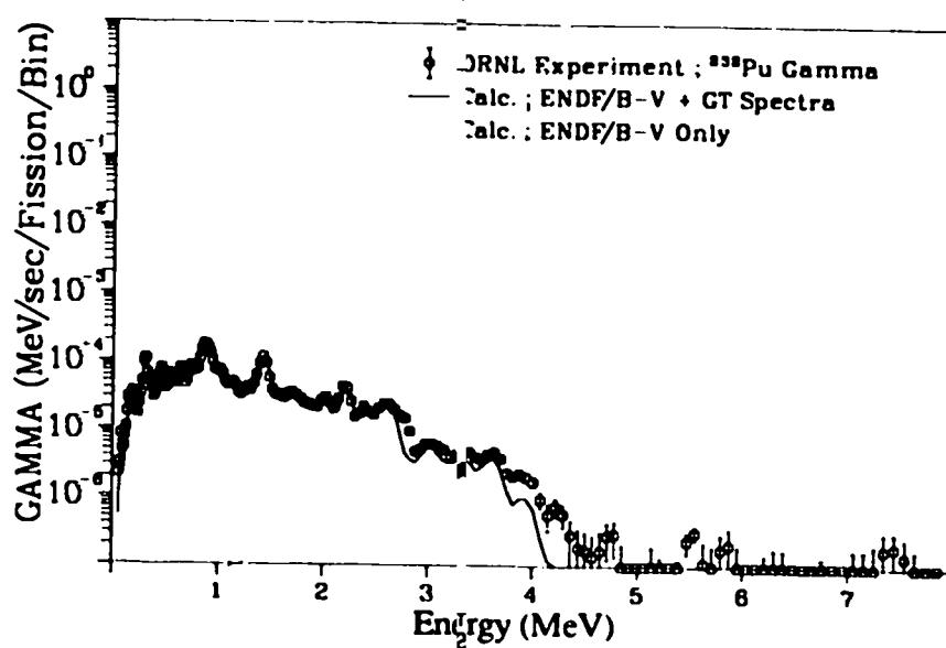
Fig. 100. Gamma spectrum after  $^{239}\text{Pu}$  thermal fission
