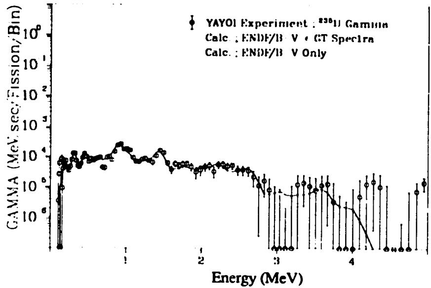
Fig. 209. Gamma spectrum after  $^{235}\text{U}$  fast neutron fission
