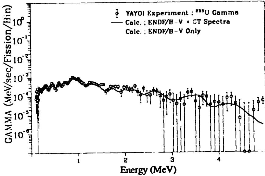
Fig. 202. Gamma spectrum after  $^{235}\text{U}$  fast neutron fission
