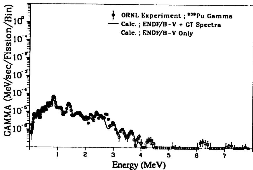
Fig. 103. Gamma spectrum after  $^{239}\text{Pu}$  thermal fission
