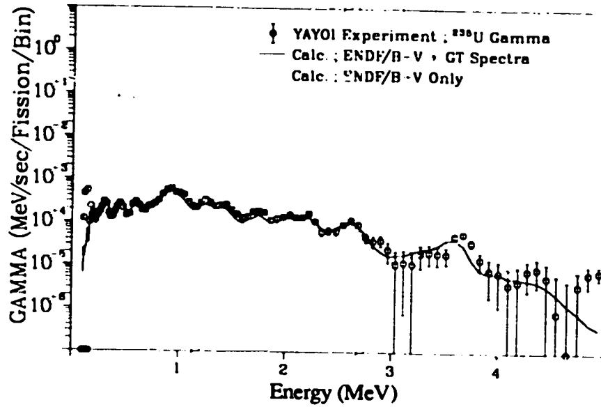
Fig. 221. Gamma spectrum after  $^{235}\text{U}$  fast neutron fission
