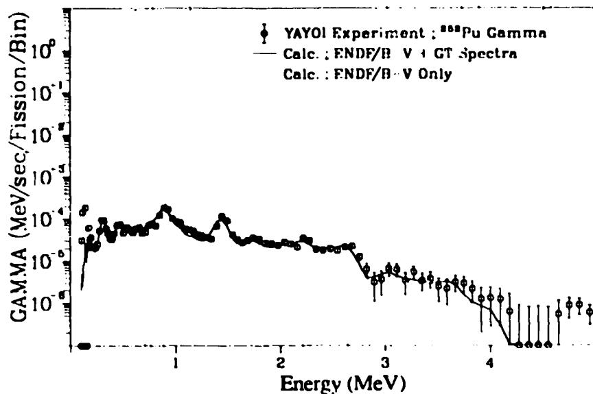
Fig. 316. Gamma spectrum after  $^{239}\text{Pu}$  fast neutron fission
