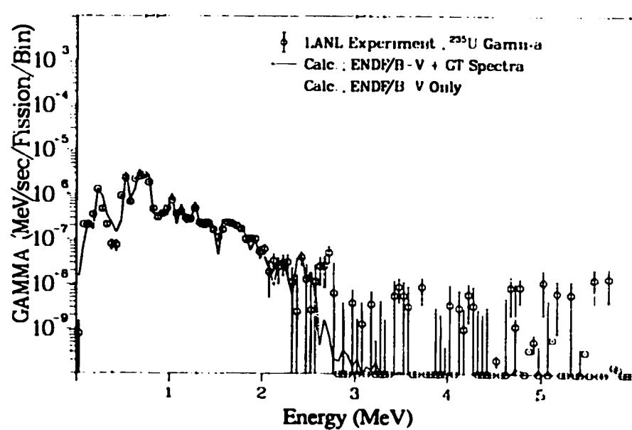
Fig. 398. Gamma spectrum after  $^{235}\text{U}$  thermal neutron fission
