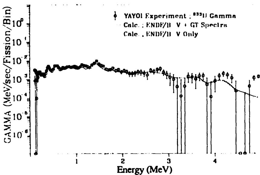
Fig. 150. Gamma spectrum after  $^{233}\text{U}$  fast neutron fission
