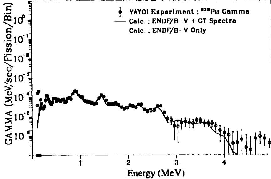
Fig. 315. Gamma spectrum after  $^{239}\text{Pu}$  fast neutron fission
