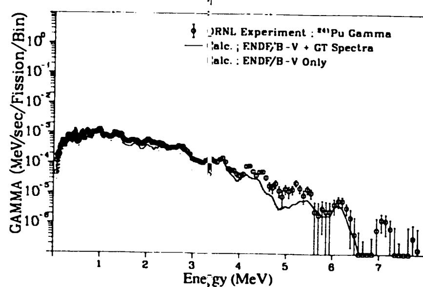
Fig. 135. Gamma spectrum after  $^{241}\text{Pu}$  thermal fission
