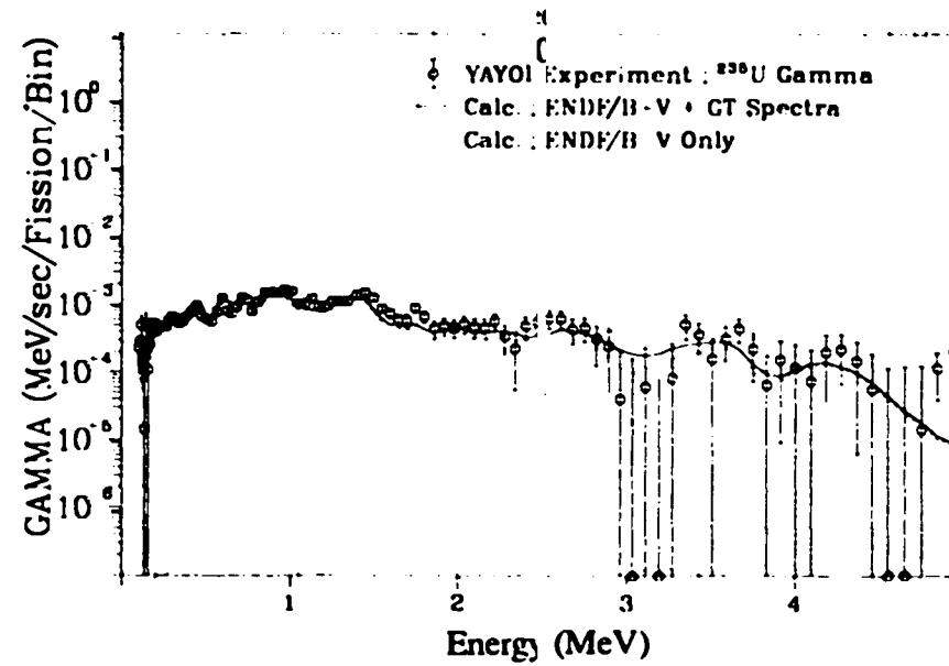
Fig. 199. Gamma spectrum after  $^{235}\text{U}$  fast neutron fission
