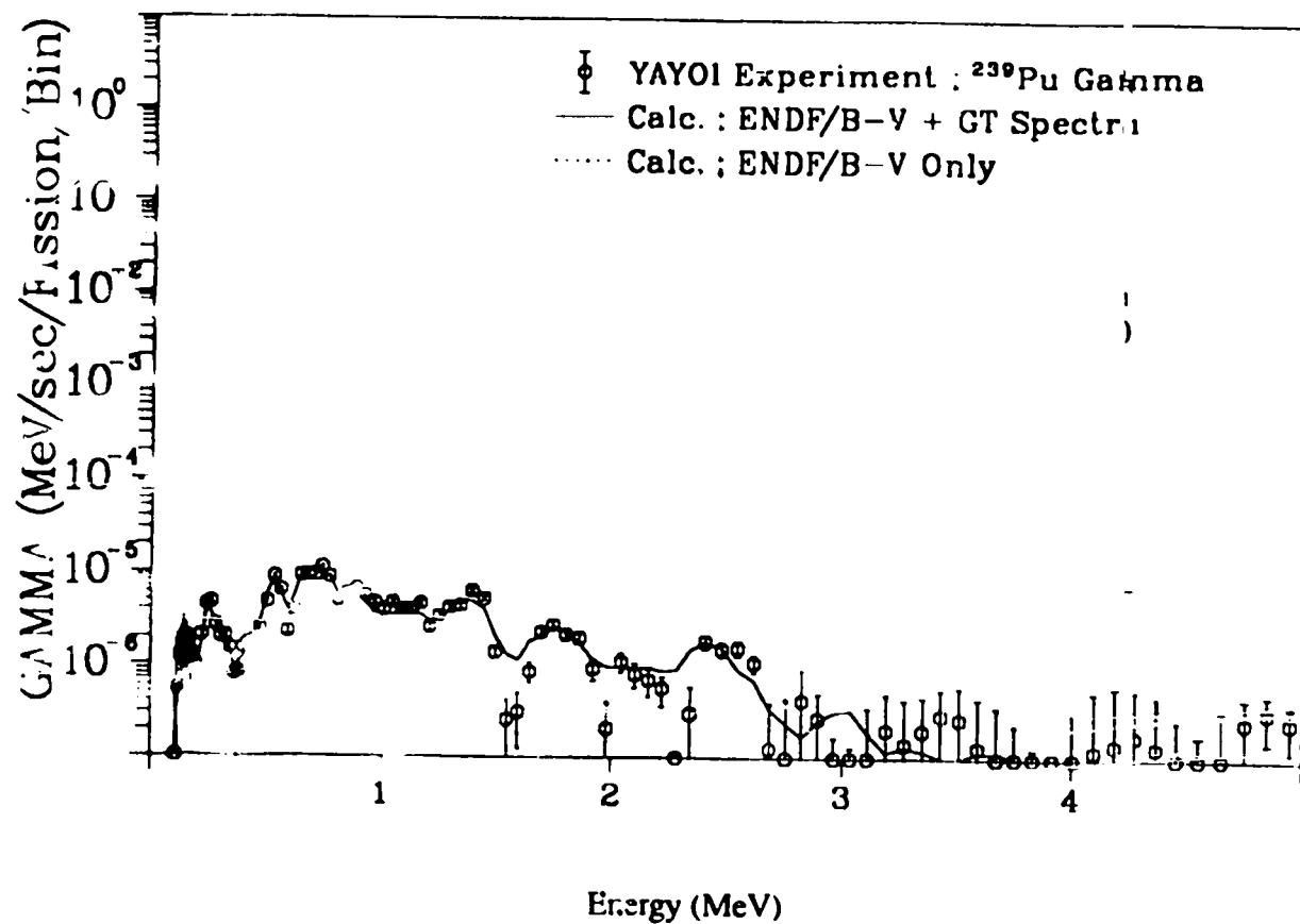
Fig. 327 Gamma spectrum after  $^{239}\text{Pu}$  fast neutron fission
