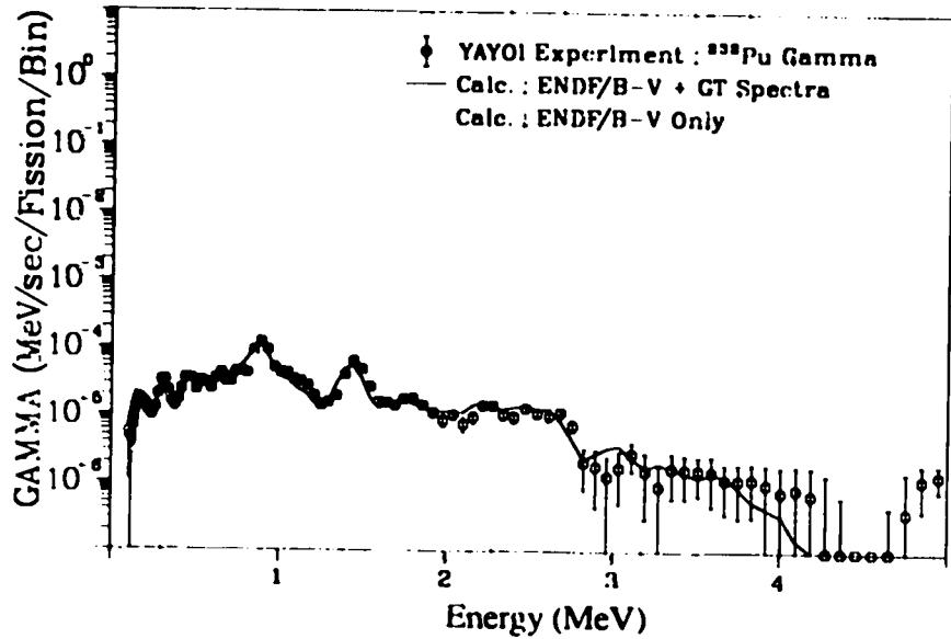
Fig. 319. Gamma spectrum after  $^{239}\text{Pu}$  fast neutron fission
