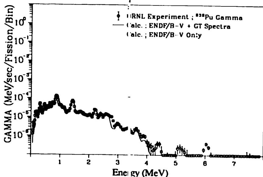
Fig. 101. Gamma spectrum after  $^{239}\text{Pu}$  thermal fission
