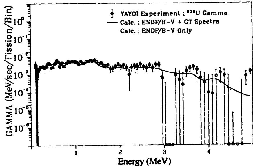
Fig. 244. Gamma spectrum after <sup>238</sup>U fast neutron fission
