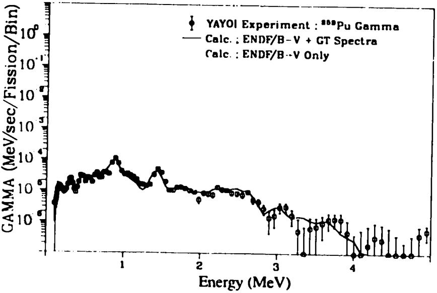
Fig. 320. Gamma spectrum after  $^{239}\text{Pu}$  fast neutron fission
