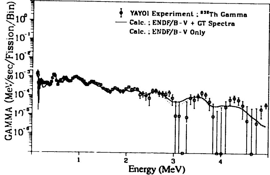
Fig. 356. Gamma spectrum after  $^{232}\text{Th}$  fast neutron fission ( $T_{\text{irrad.}} = 100.0$  sec,  $T_{\text{cool.}} = 550.0$  sec).
