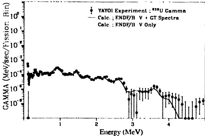
Fig. 272. Gamma spectrum after  $^{238}\text{U}$  fast neutron fission
