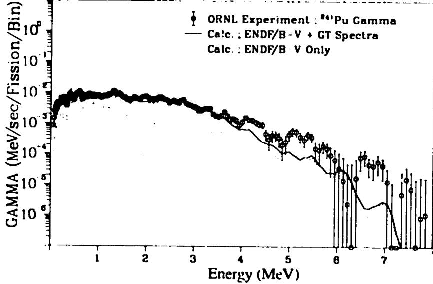
Fig. 113. Gamma spectrum after  $^{241}\text{Pu}$  thermal fission
