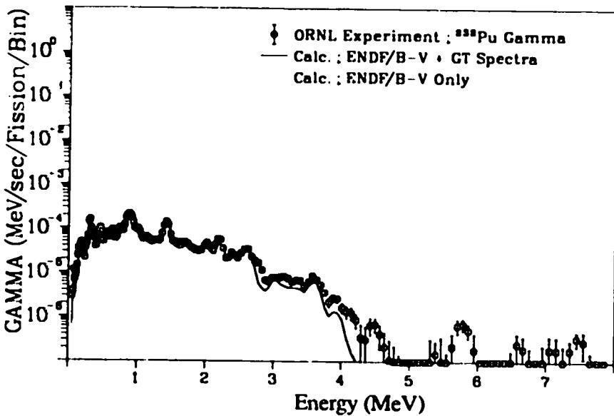
Fig. 99. Gamma spectrum after  $^{239}\text{Pu}$  thermal fission
