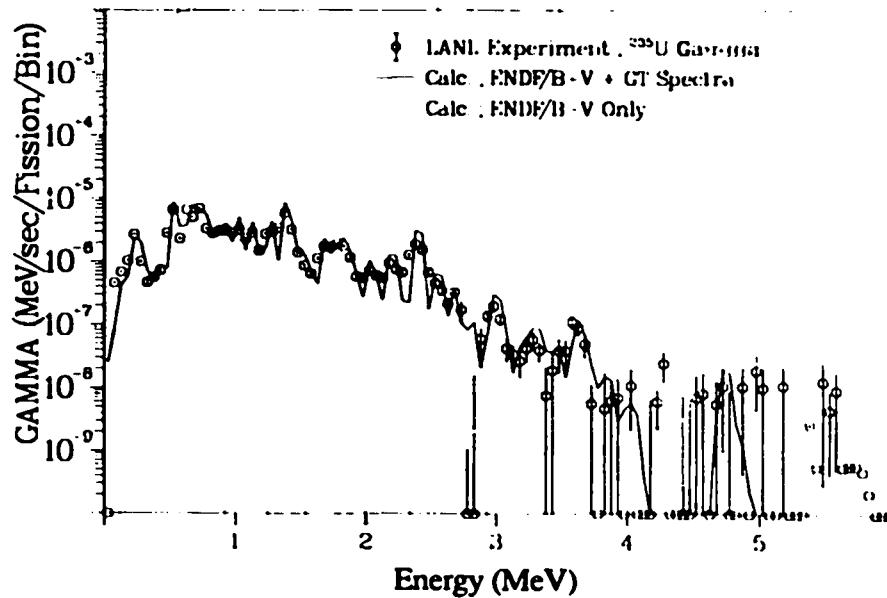
Fig. 396. Gamma spectrum after  $^{235}\text{U}$  thermal neutron fission
