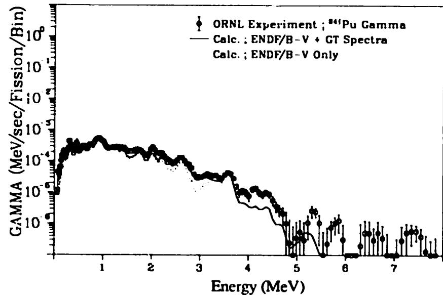
Fig. 138. Gamma spectrum after  $^{241}\text{Pu}$  thermal fission
