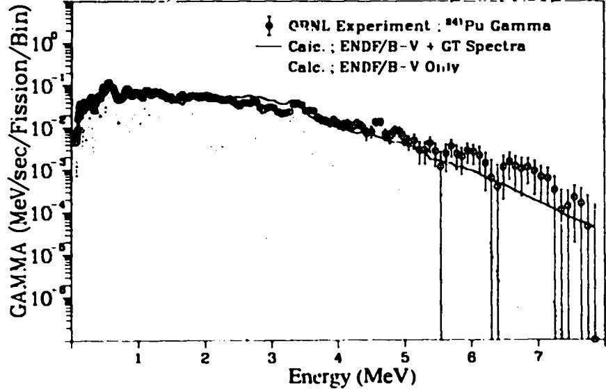
Fig. 105. Gamma spectrum after  $^{241}\text{Pu}$  thermal fission
