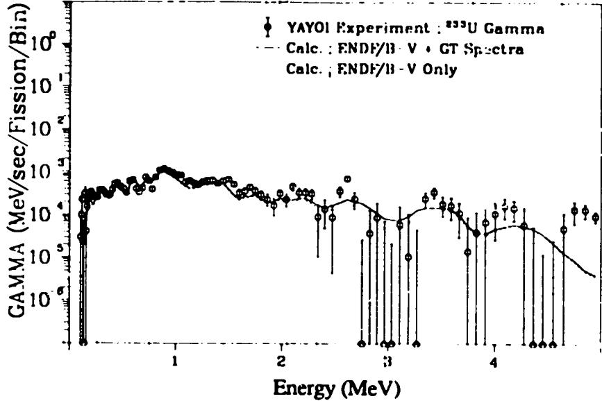
Fig. 157. Gamma spectrum after  $^{233}\text{U}$  fast neutron fission
