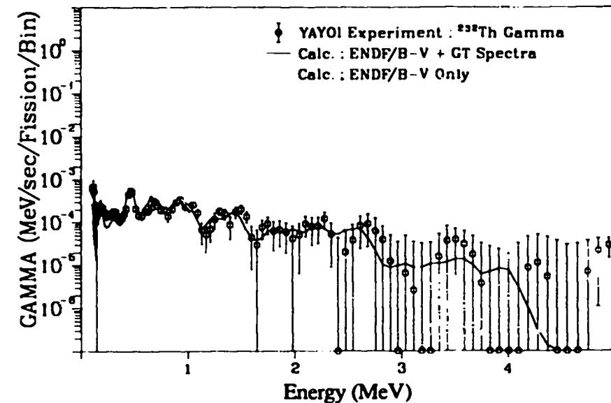
Fig. 347. Gamma spectrum after  $^{232}\text{Th}$  fast neutron fission
