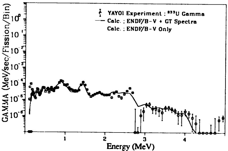
Fig. 178. Gamma spectrum after  $^{233}\text{U}$  fast neutron fission
