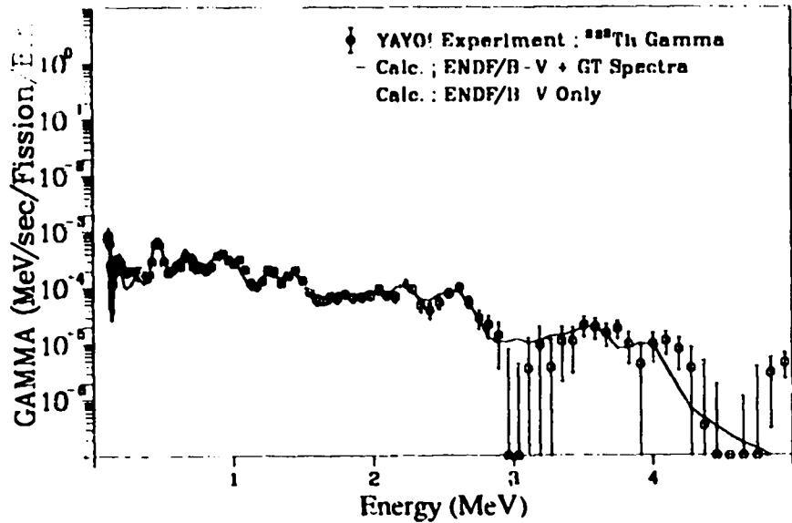
Fig. 360. Gamma spectrum after  $^{232}\text{Th}$  fast neutron fission
