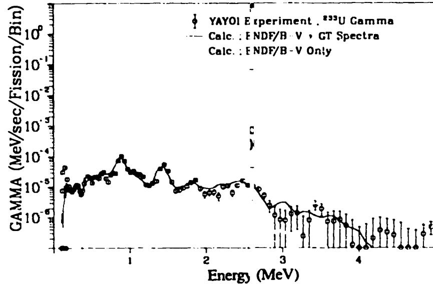
Fig. 232. Gamma spectrum after  $^{235}\text{U}$  fast neutron fission
