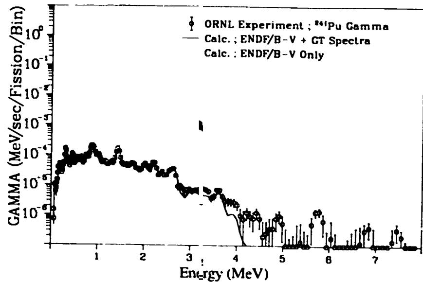
Fig. 143. Gamma spectrum after  $^{241}\text{Pu}$  thermal fission
