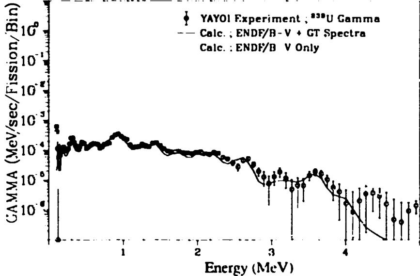
Fig. 271. Gamma spectrum after  $^{238}\text{U}$  fast neutron fission
