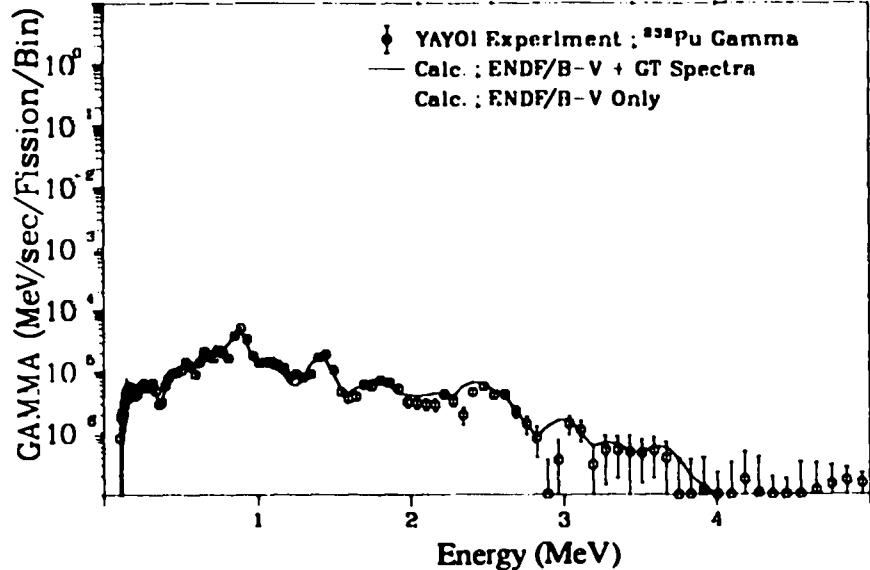
Fig. 323. Gamma spectrum after  $^{239}\text{Pu}$  fast neutron fission
