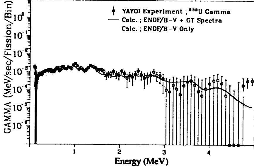
Fig. 248. Gamma spectrum after  $^{238}\text{U}$  fast neutron fission
