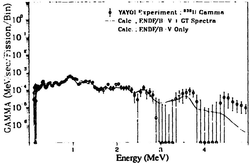
Fig. 205. Gamma spectrum after  $^{235}\text{U}$  fast neutron fission ( $T_{\text{irrad.}} = 10.0 \text{ sec}$ ,  $T_{\text{cool.}} = 900.0 \text{ sec}$ ).
