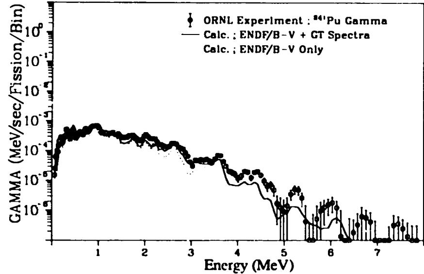
Fig. 137. Gamma spectrum after  $^{241}\text{Pu}$  thermal fission
