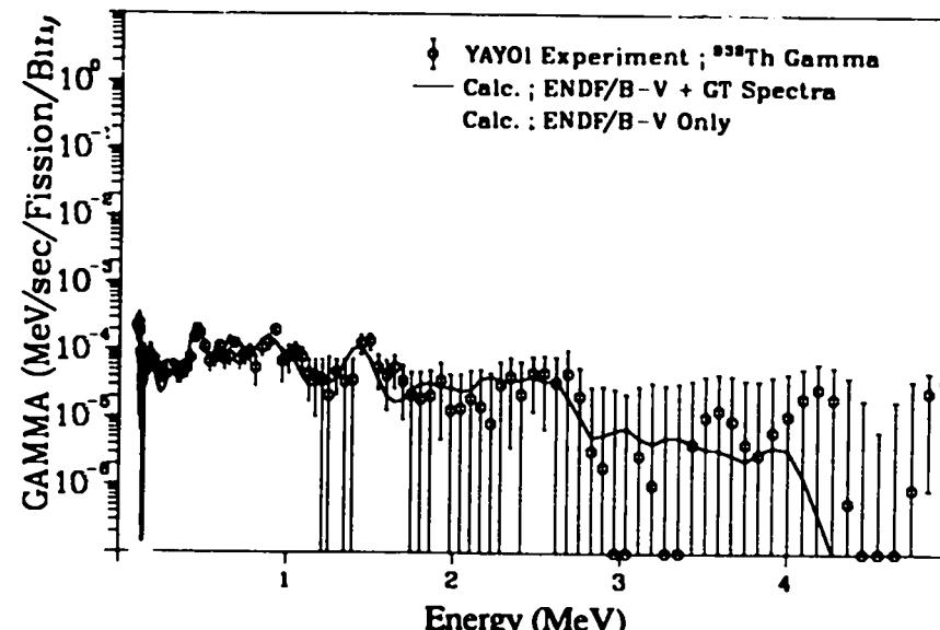
Fig. 351. Gamma spectrum after  $^{232}\text{Th}$  fast neutron fission
