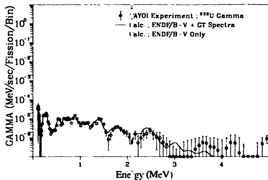
Fig. 285. Gamma spectrum after  $^{238}\text{U}$  fast neutron fission
