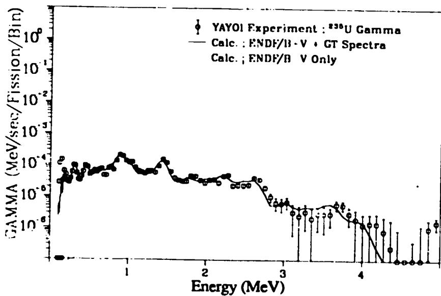
Fig. 226. Gamma spectrum after  $^{235}\text{U}$  fast neutron fission
