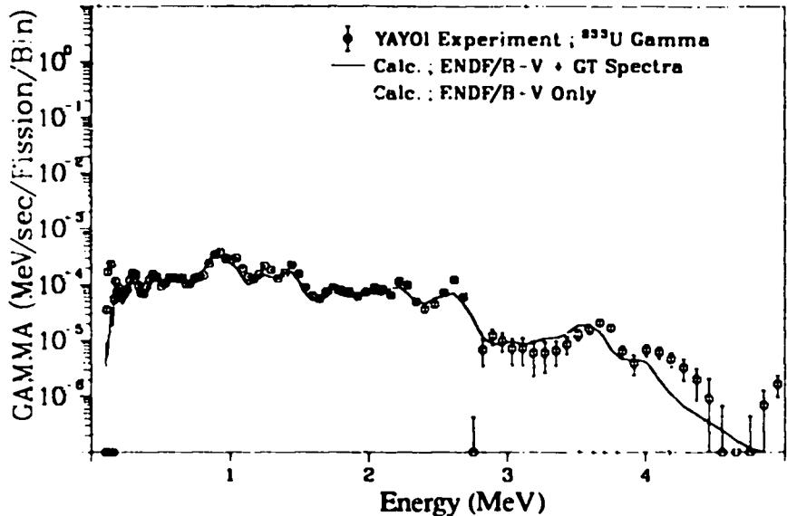
Fig. 173. Gamma spectrum after  $^{233}\text{U}$  fast neutron fission ( $T_{\text{irrad.}} = 100.0$  sec,  $T_{\text{cool.}} = 1600.0$  sec).
