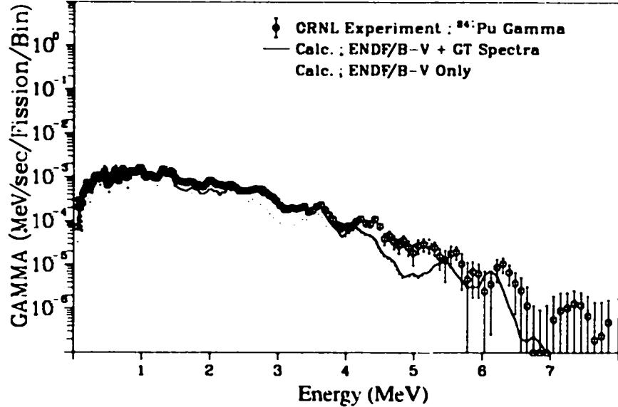
Fig. 129. Gamma spectrum after  $^{241}\text{Pu}$  thermal fission
