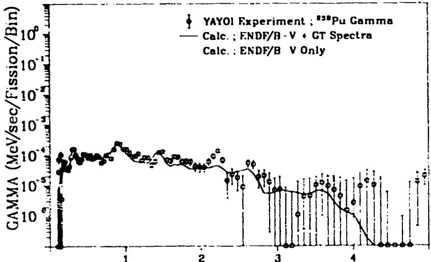
Fig. 307. Gamma spectrum after  $^{239}\text{Pu}$  fast neutron fission
