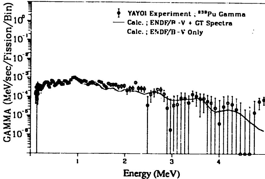
Fig. 299. Gamma spectrum after  $^{239}\text{Pu}$  fast neutron fission
