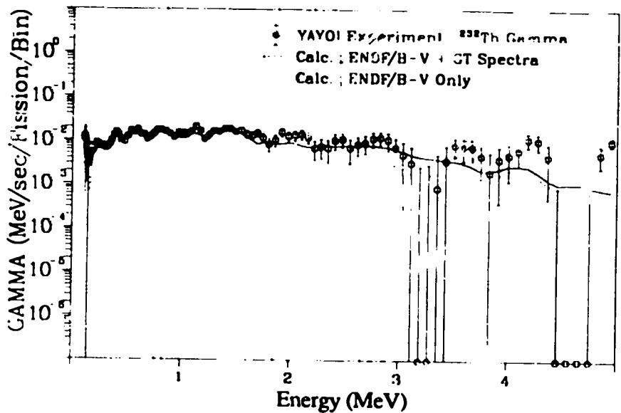
Fig. 329. Gamma spectrum after  $^{232}\text{Th}$  fast neutron fission
