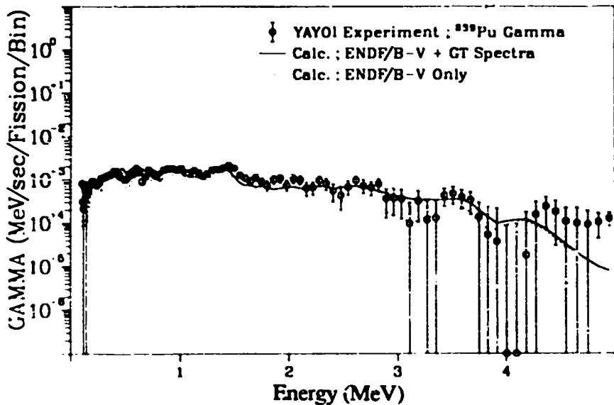
Fig. 295. Gamma spectrum after  $^{239}\text{Pu}$  fast neutron fission
