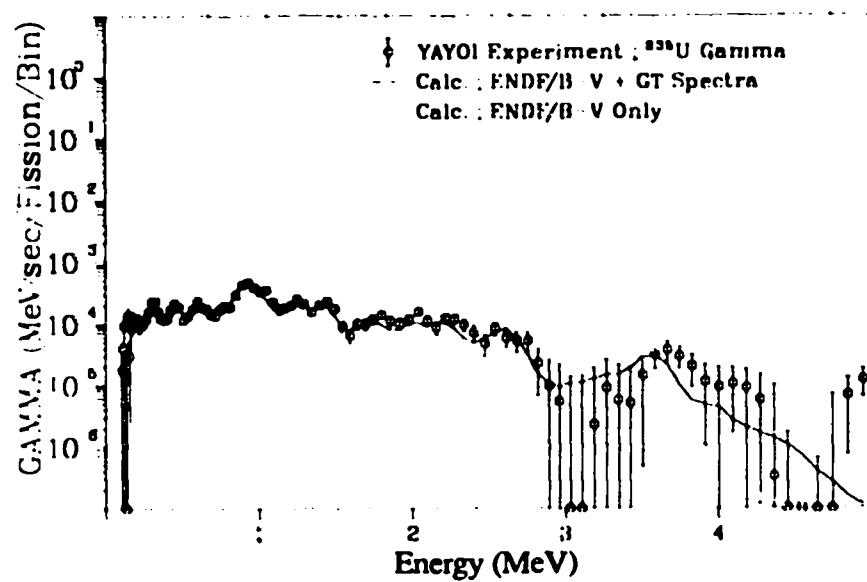
Fig. 206. Gamma spectrum after  $^{235}\text{U}$  fast neutron fission ( $T_{\text{irrad.}} = 10.0 \text{ sec}$ ,  $T_{\text{cool.}} = 1200.0 \text{ sec}$ ).
