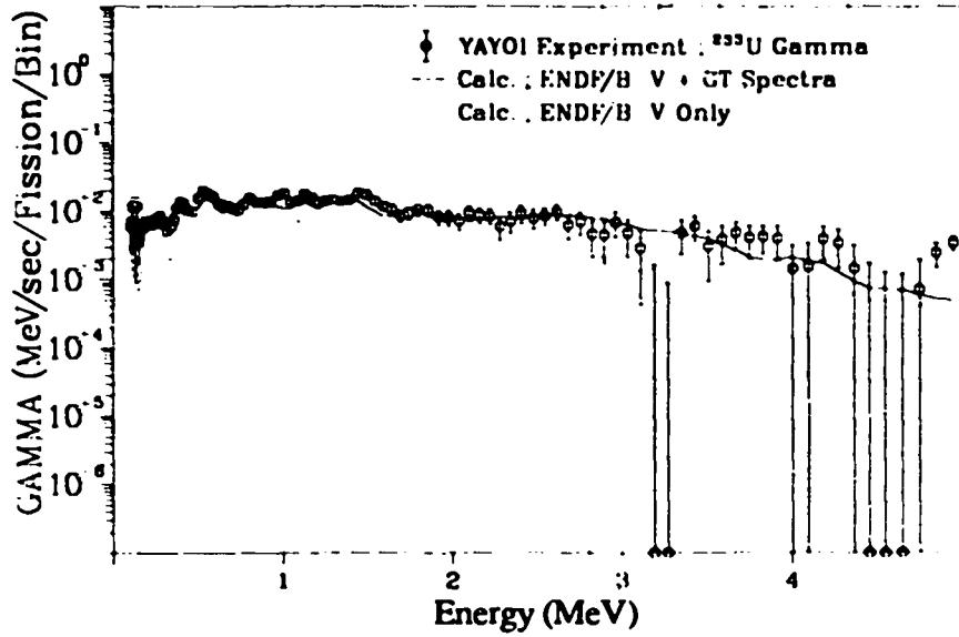
Fig. 189. Gamma spectrum after  $^{235}\text{U}$  fast neutron fission
