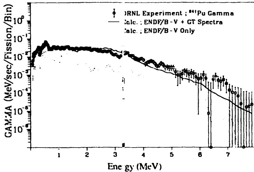
Fig. 108. Gamma spectrum after  $^{241}\text{Pu}$  thermal fission
