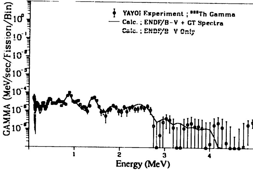
Fig. 368. Gamma spectrum after  $^{232}\text{Th}$  fast neutron fission
