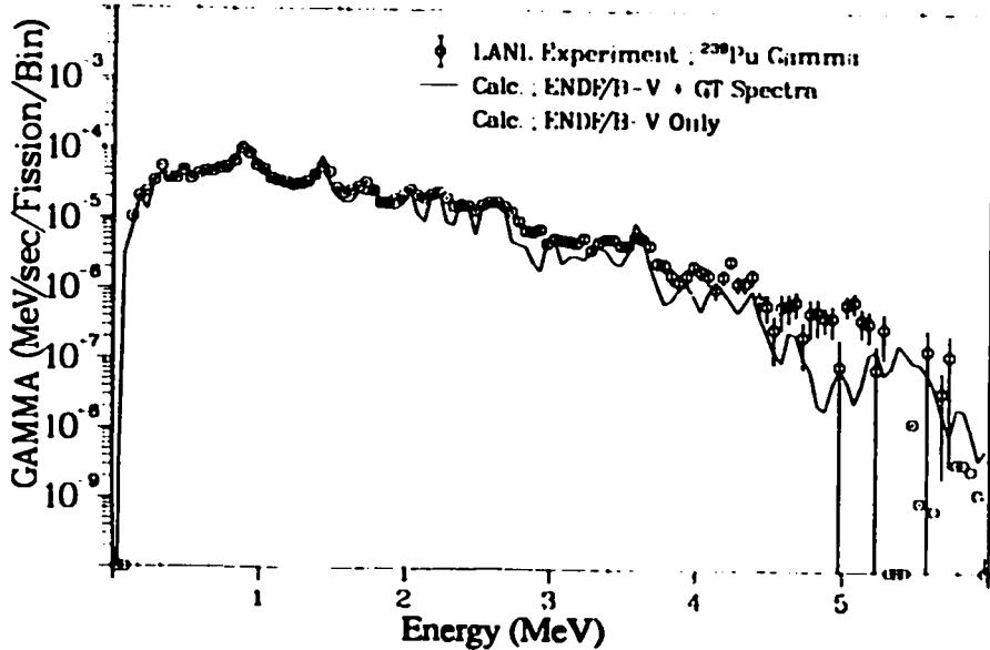
Fig. 401. Gamma spectrum after  $^{239}\text{Pu}$  thermal neutron fission
