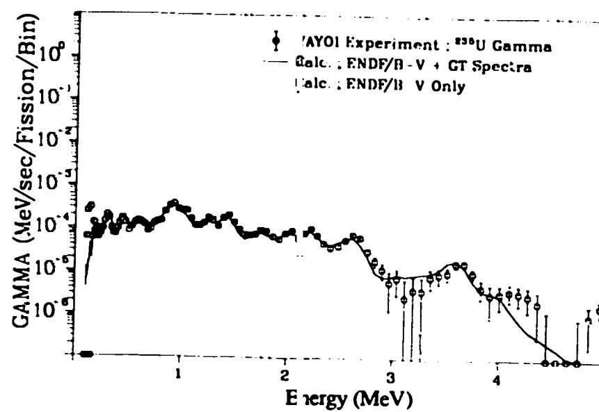
Fig. 223. Gamma spectrum after  $^{235}\text{U}$  fast neutron fission
