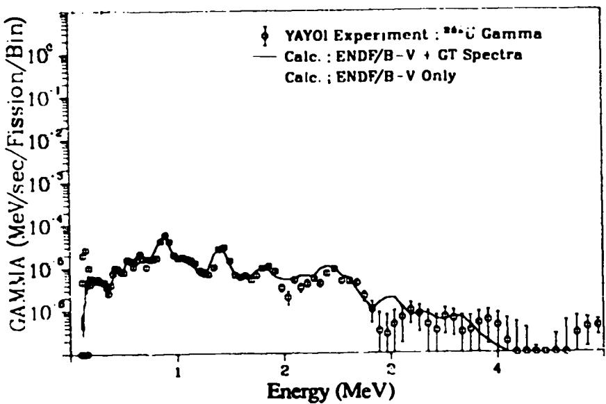
Fig. 234. Gamma spectrum after  $^{235}\text{U}$  fast neutron fission
