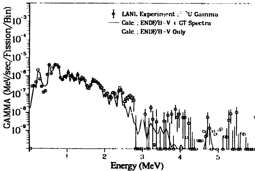
Fig. 397. Gamma spectrum after  $^{235}\text{U}$  thermal neutron fission
