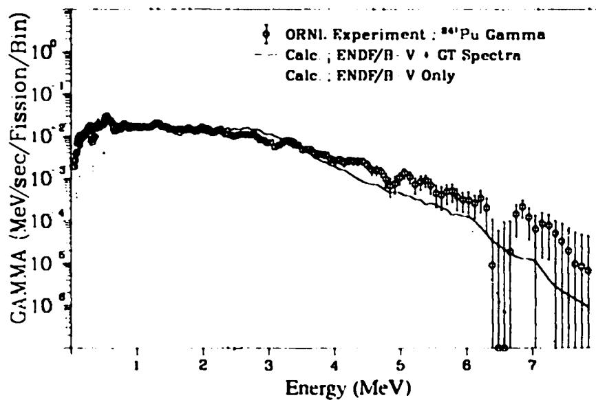
Fig. 110. Gamma spectrum after  $^{241}\text{Pu}$  thermal fission
