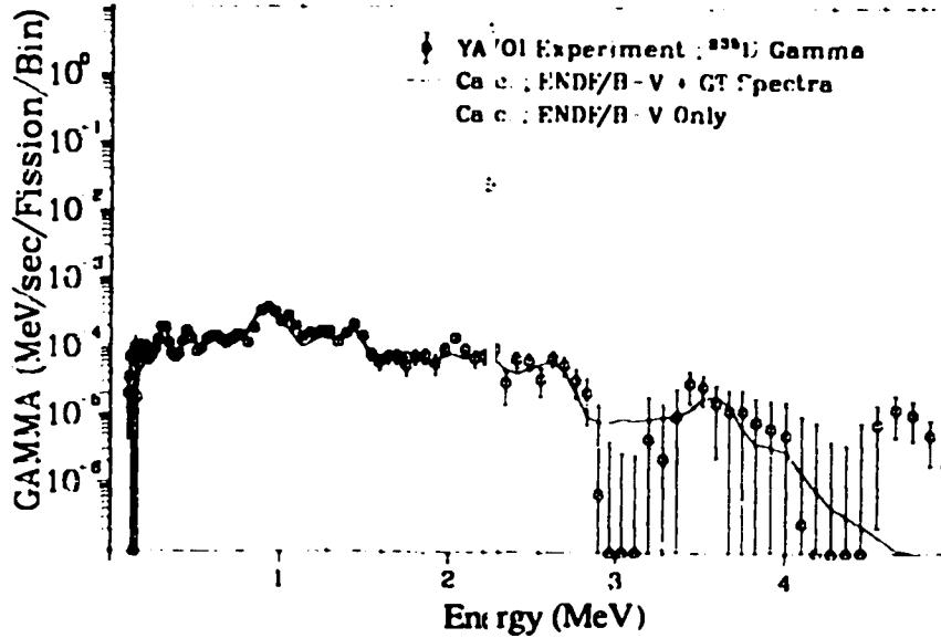
Fig. 207. Gamma spectrum after  $^{235}\text{U}$  fast neutron fission ( $T_{\text{irrad.}} = 10.0 \text{ sec}$ ,  $T_{\text{cool.}} = 1600.0 \text{ sec}$ ).
