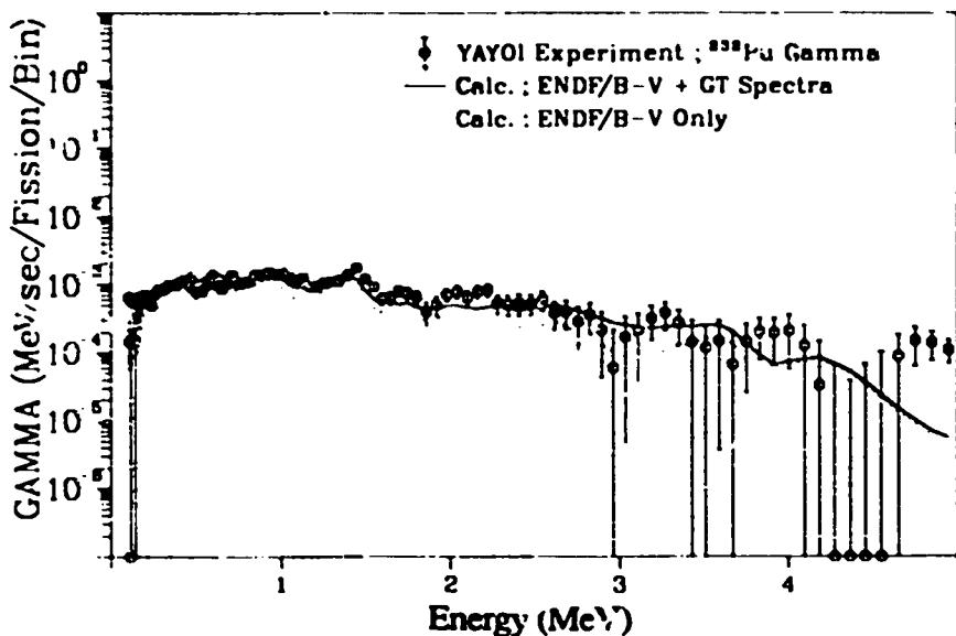
Fig. 296. Gamma spectrum after  $^{239}\text{Pu}$  fast neutron fission
