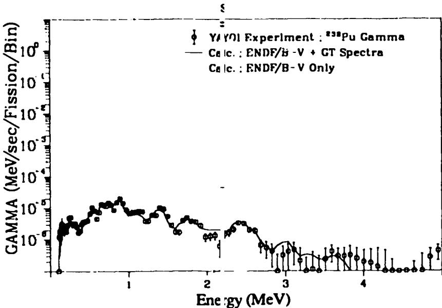
Fig. 325. Gamma spectrum after  $^{239}\text{Pu}$  fast neutron fission
