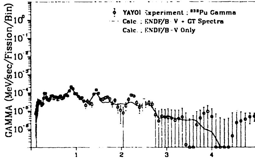
Fig. 309. Gamma spectrum after  $^{239}\text{Pu}$  fast neutron fission
