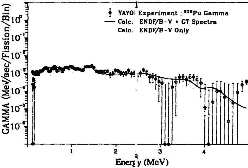
Fig. 294. Gamma spectrum after  $^{239}\text{Pu}$  fast neutron fission
