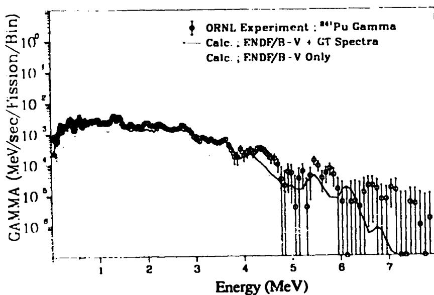
Fig. 118. Gamma spectrum after  $^{241}\text{Pu}$  thermal fission
