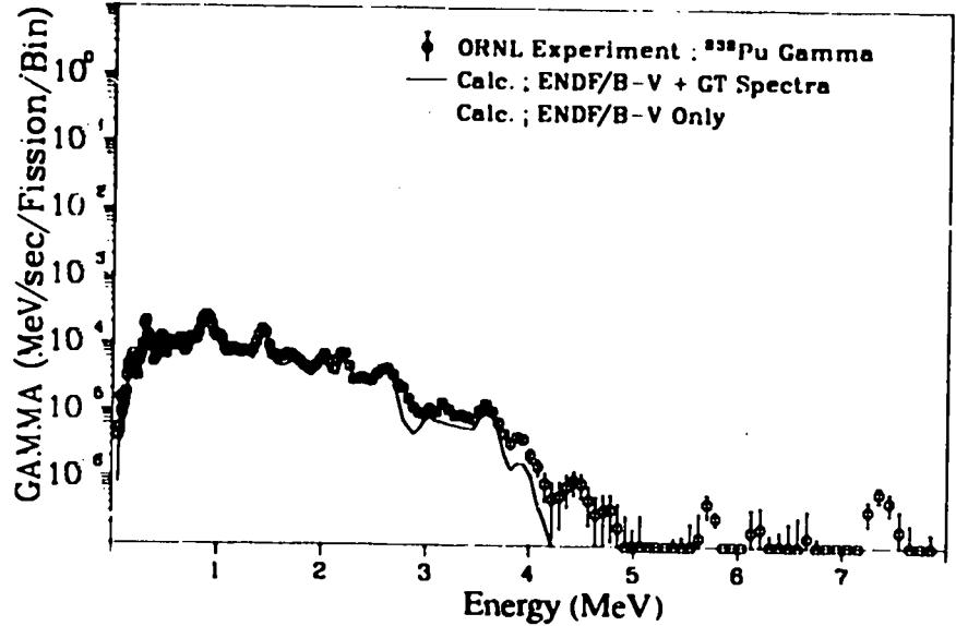
Fig. 98. Gamma spectrum after  $^{239}\text{Pu}$  thermal fission
