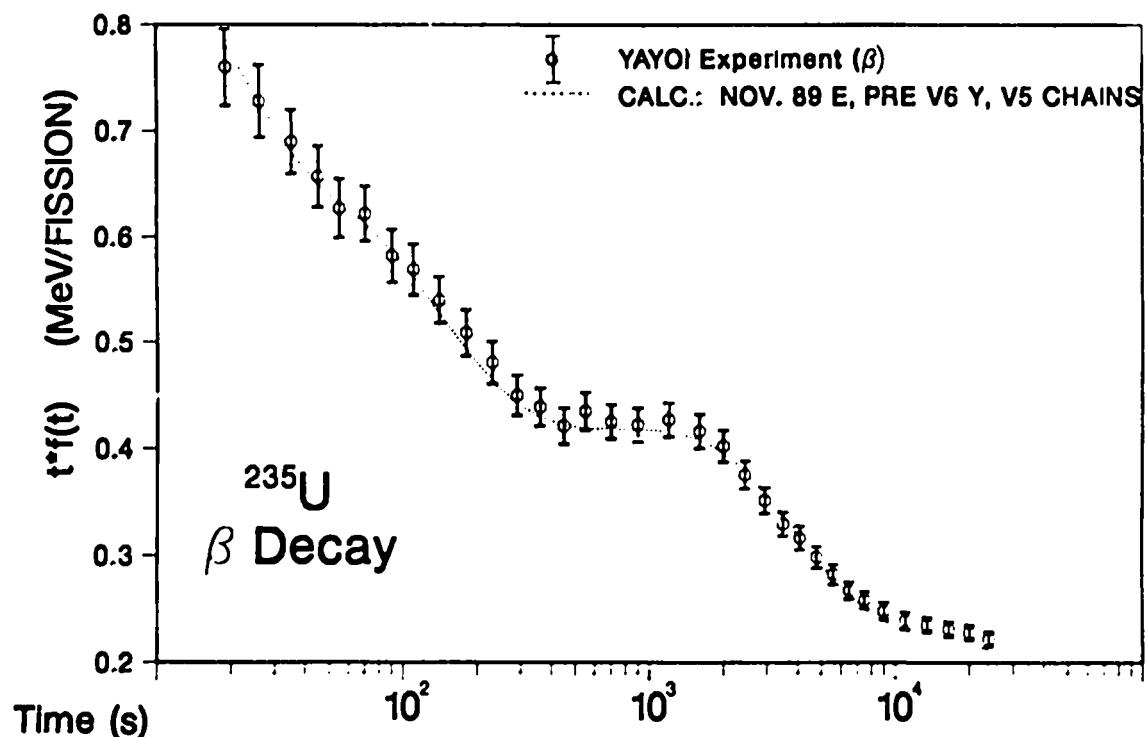
Fig. C-2. Beta decay energy after  $^{235}\text{U}$  fast fission (pulse).
