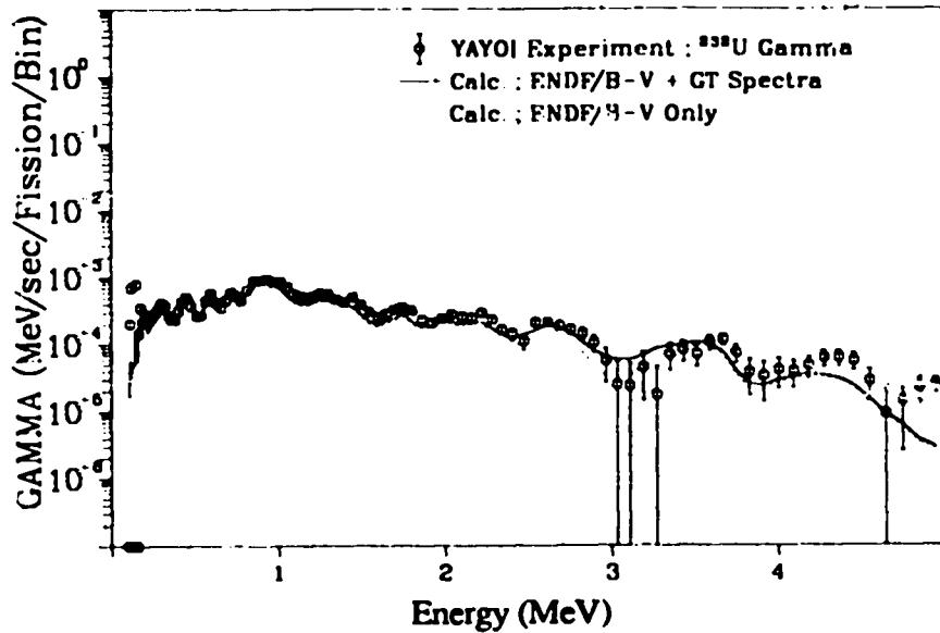
Fig. 218. Gamma spectrum after  $^{235}\text{U}$  fast neutron fission
