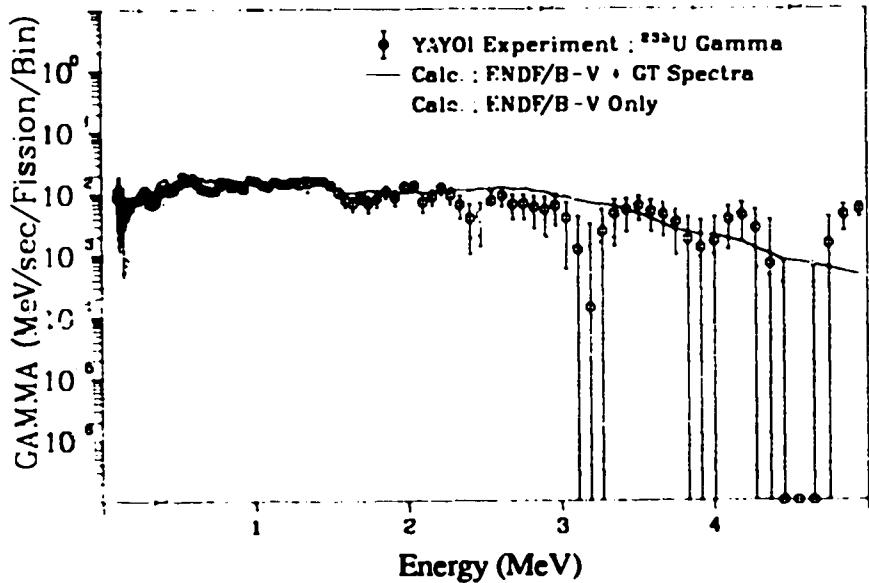
Fig. 239. Gamma spectrum after  $^{238}\text{U}$  fast neutron fission
