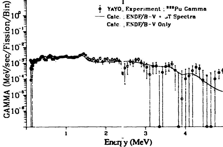
Fig. 293. Gamma spectrum after  $^{239}\text{Pu}$  fast neutron fission
