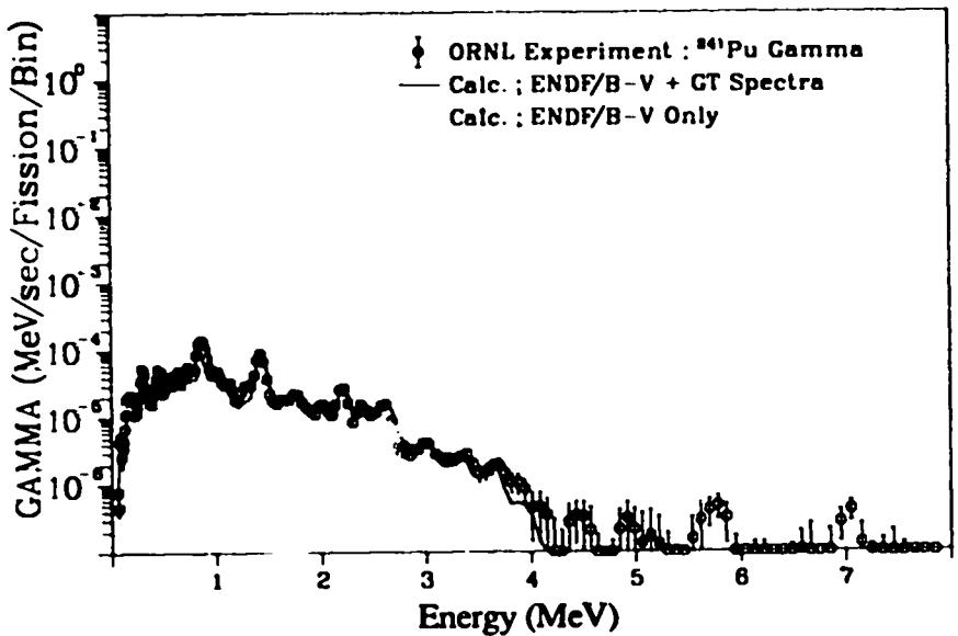
Fig. 145. Gamma spectrum after  $^{241}\text{Pu}$  thermal fission
