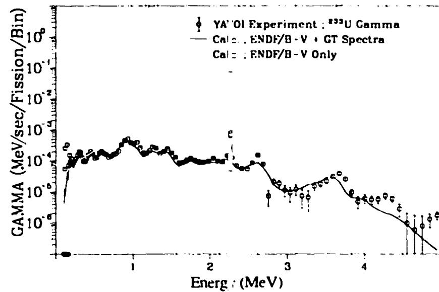
Fig. 172. Gamma spectrum after  $^{233}\text{U}$  fast neutron fission
