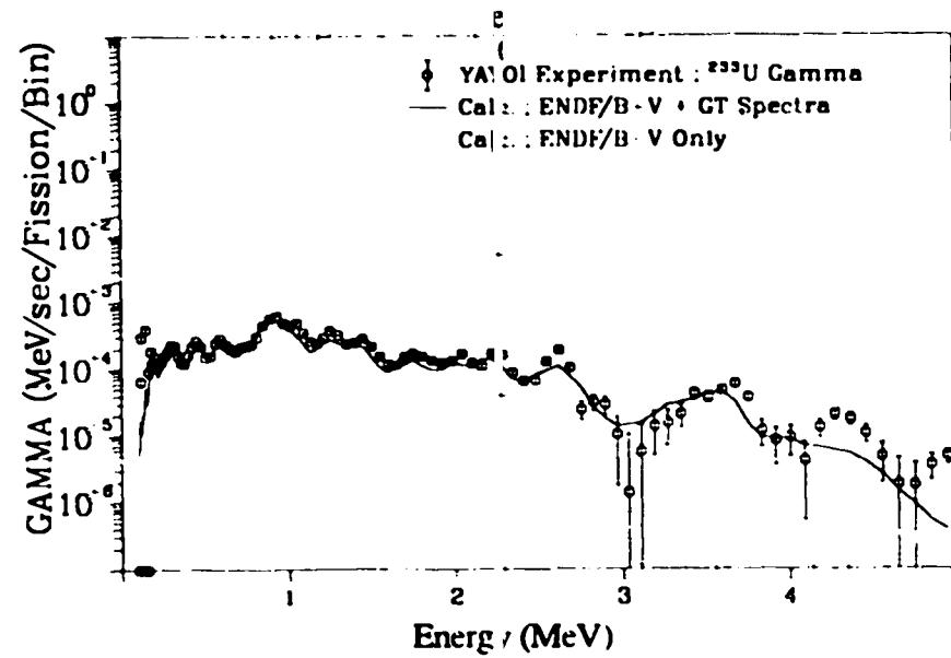
Fig. 171. Gamma spectrum after  $^{233}\text{U}$  fast neutron fission
