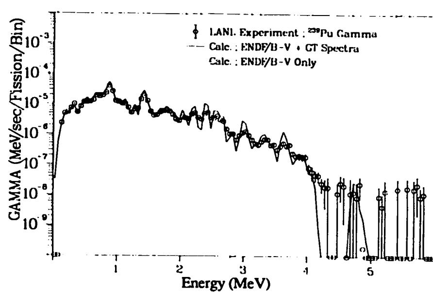
Fig. 406. Gamma spectrum after  $^{239}\text{Pu}$  thermal neutron fission
