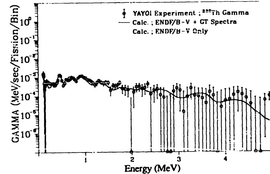
Fig. 341. Gamma spectrum after  $^{232}\text{Th}$  fast neutron fission ( $T_{\text{irrad.}} = 10.0$  sec,  $T_{\text{cool.}} = 450.0$  sec).
