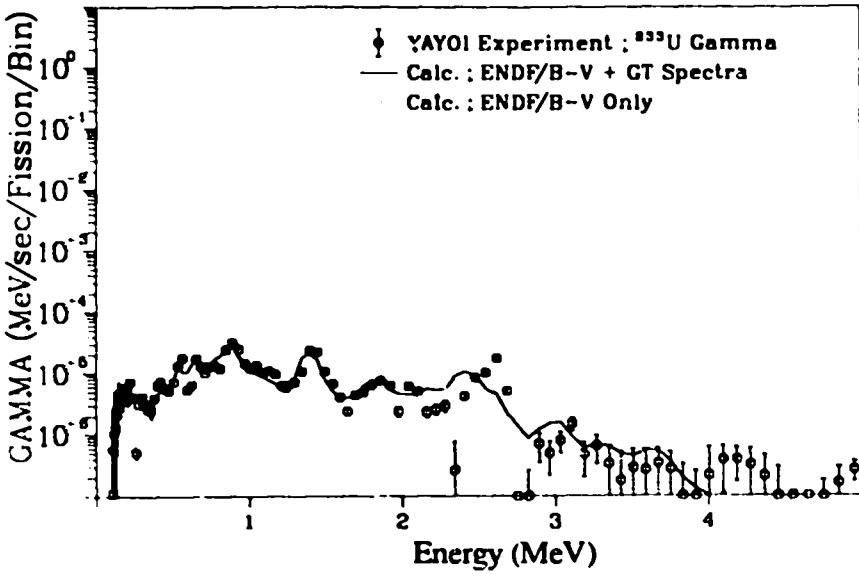
Fig. 185. Gamma spectrum after  $^{233}\text{U}$  fast neutron fission
