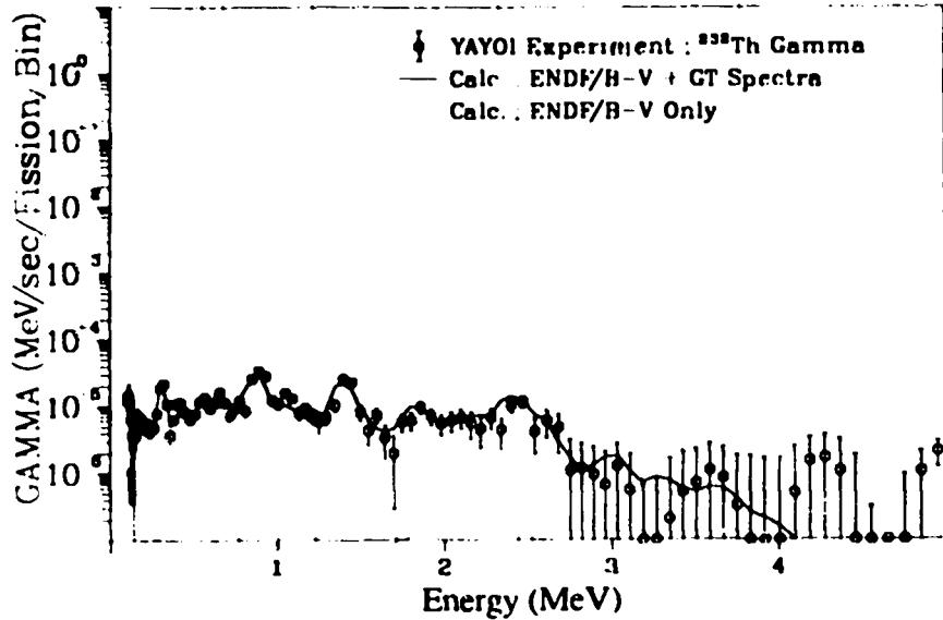
Fig. 372. Gamma spectrum after  $^{232}\text{Th}$  fast neutron fission
