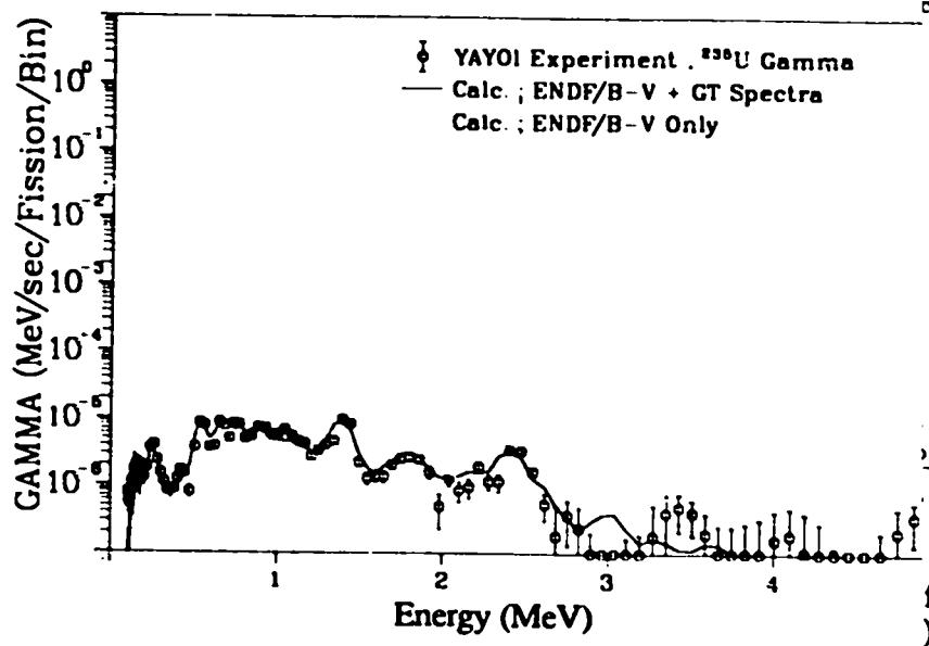
Fig. 238. Gamma spectrum after  $^{235}\text{U}$  fast neutron fission
