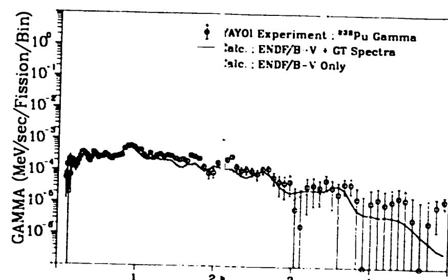
Fig. 302. Gamma spectrum after  $^{239}\text{Pu}$  fast neutron fission
