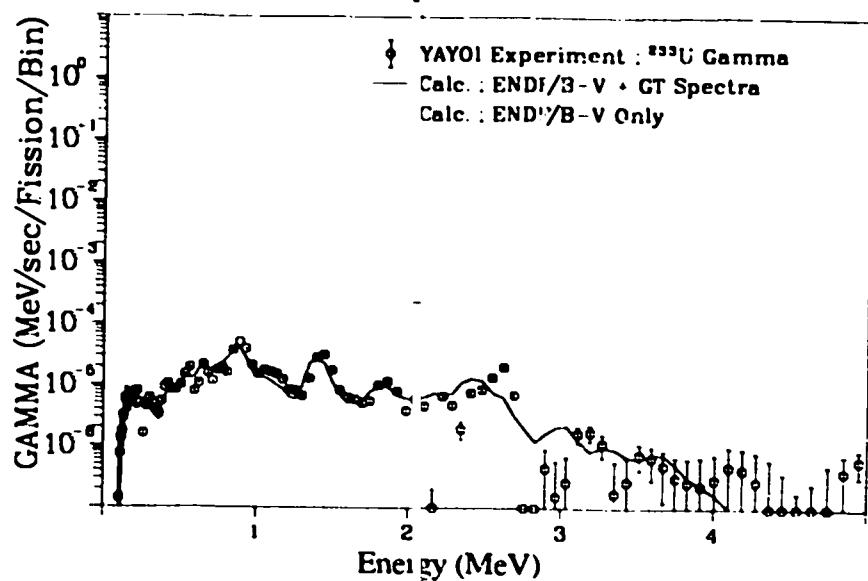
Fig. 184. Gamma spectrum after  $^{233}\text{U}$  fast neutron fission
