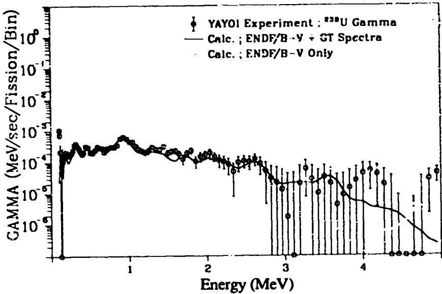
Fig. 255. Gamma spectrum after  $^{238}\text{U}$  fast neutron fission
