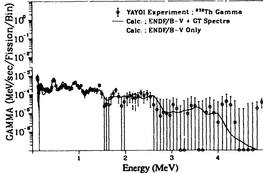
Fig. 346. Gamma spectrum after  $^{232}\text{Th}$  fast neutron fission
