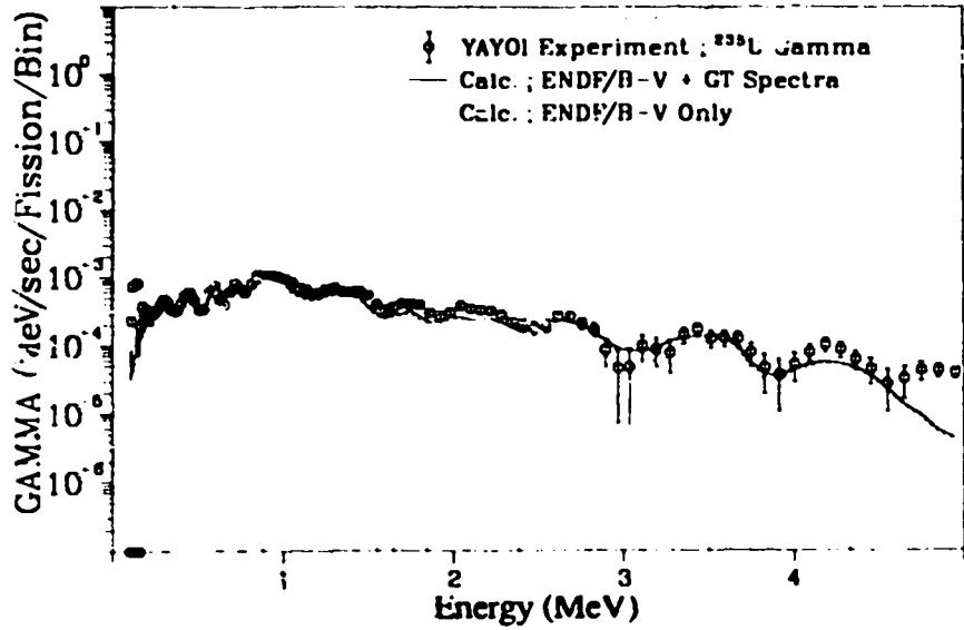
Fig. 217. Gamma spectrum after  $^{235}\text{U}$  fast neutron fission
