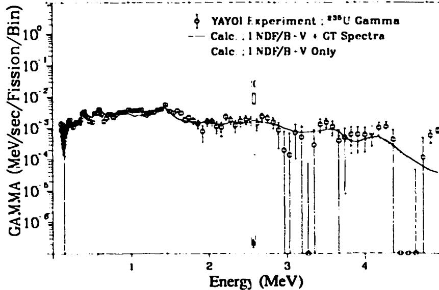
Fig. 195. Gamma spectrum after  $^{235}\text{U}$  fast neutron fission
