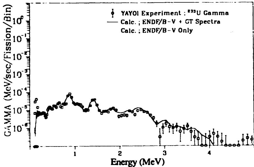
Fig. 233. Gamma spectrum after  $^{235}\text{U}$  fast neutron fission
