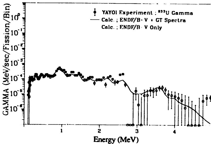
Fig. 162. Gamma spectrum after  $^{233}\text{U}$  fast neutron fission
