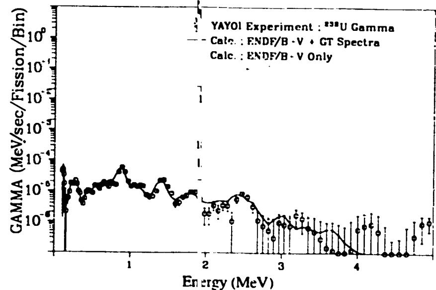
Fig. 282. Gamma spectrum after  $^{238}\text{U}$  fast neutron fission
