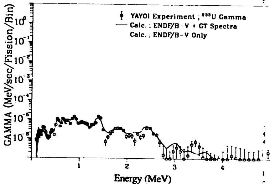
Fig. 237. Gamma spectrum after  $^{235}\text{U}$  fast neutron fission
