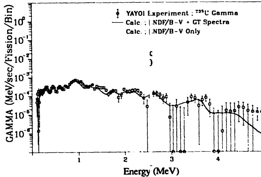
Fig. 204. Gamma spectrum after  $^{235}\text{U}$  fast neutron fission
