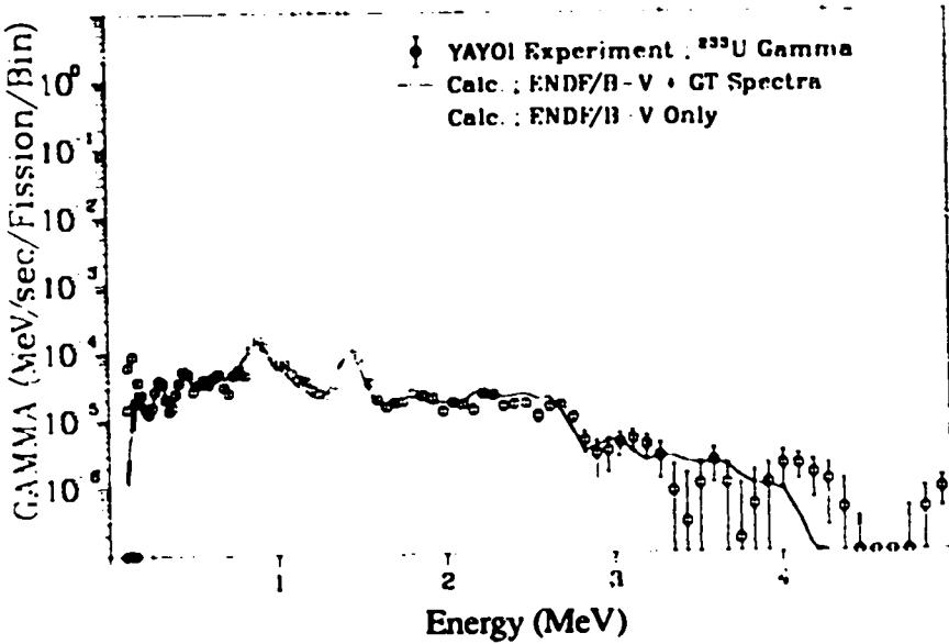
Fig. 229. Gamma spectrum after  $^{235}\text{U}$  fast neutron fission
