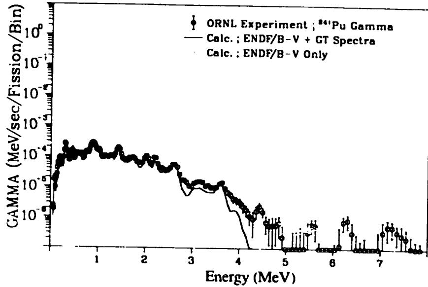
Fig. 141. Gamma spectrum after  $^{241}\text{Pu}$  thermal fission
