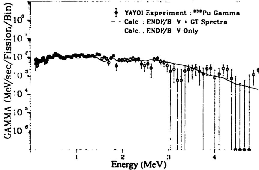
Fig. 287. Gamma spectrum after  $^{239}\text{Pu}$  fast neutron fission ( $T_{\text{irrad.}} = 10.0 \text{ sec.}$ ,  $T_{\text{cool.}} = 19.0 \text{ sec.}$ ).
