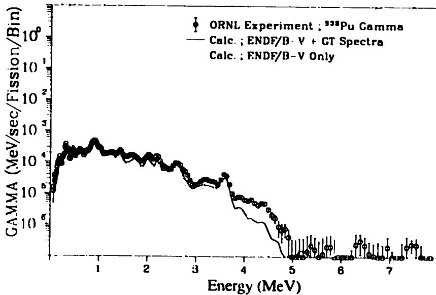
Fig. 95. Gamma spectrum after  $^{239}\text{Pu}$  thermal fission
