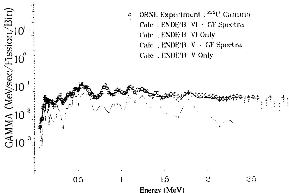
Fig. A-2. Gamma spectrum after  $^{235}\text{U}$  thermal neutron fission ( $T_{\text{irrad.}} = 1.0$  sec,  $T_{\text{cool.}} = 2.2$  sec)
