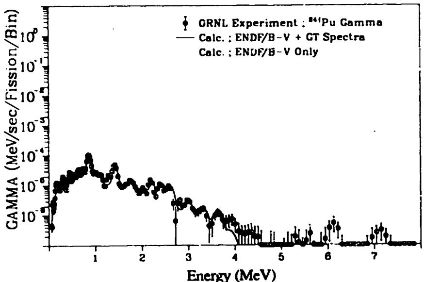
Fig. 146. Gamma spectrum after  $^{241}\text{Pu}$  thermal fission
