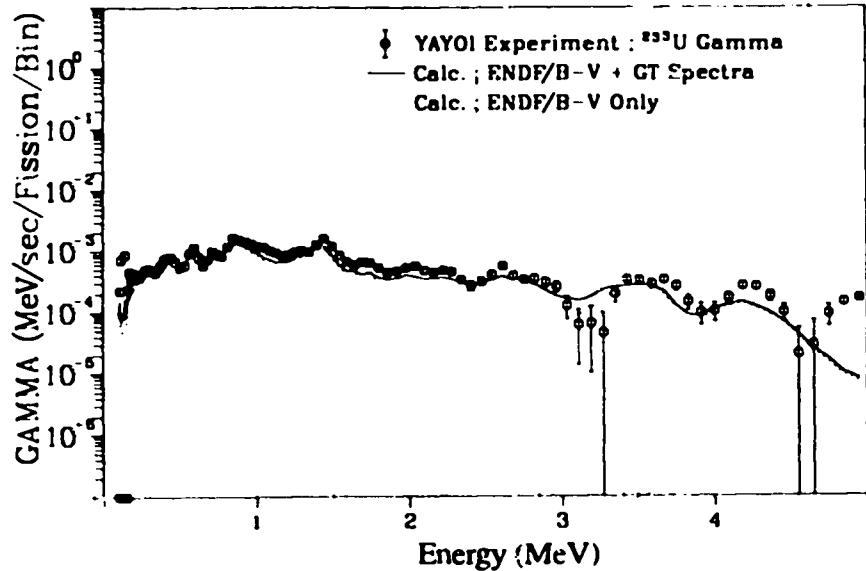
Fig. 169. Gamma spectrum after  $^{233}\text{U}$  fast neutron fission
