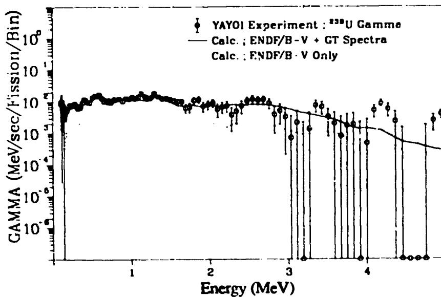
Fig. 240. Gamma spectrum after  $^{238}\text{U}$  fast neutron fission
