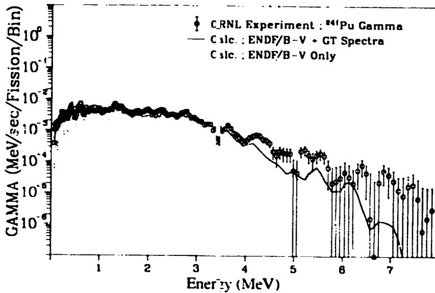
Fig. 115. Gamma spectrum after  $^{241}\text{Pu}$  thermal fission
