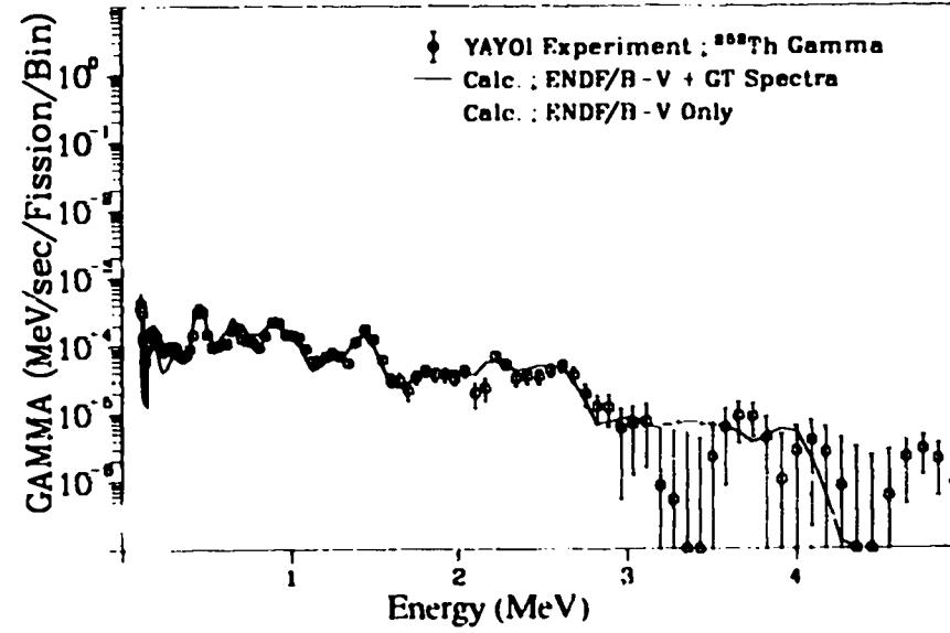
Fig. 363. Gamma spectrum after  $^{232}\text{Th}$  fast neutron fission
