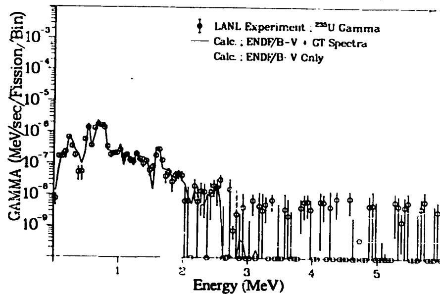
Fig. 399. Gamma spectrum after  $^{235}\text{U}$  thermal neutron fission
