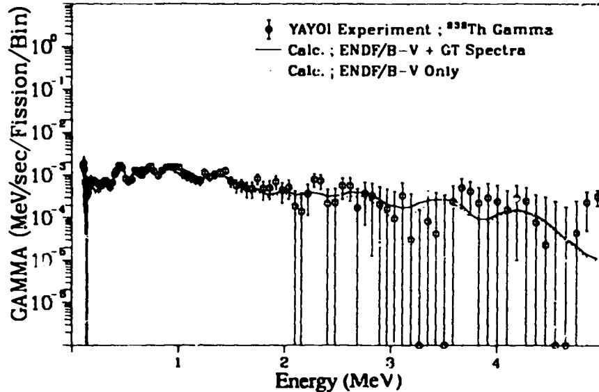
Fig. 339. Gamma spectrum after  $^{232}\text{Th}$  fast neutron fission
