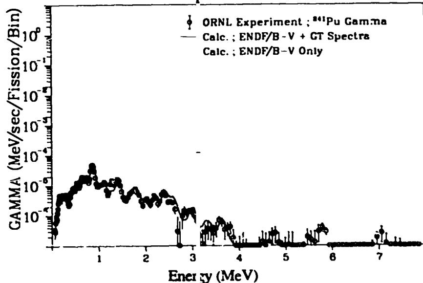
Fig. 148. Gamma spectrum after  $^{241}\text{Pu}$  thermal fission
