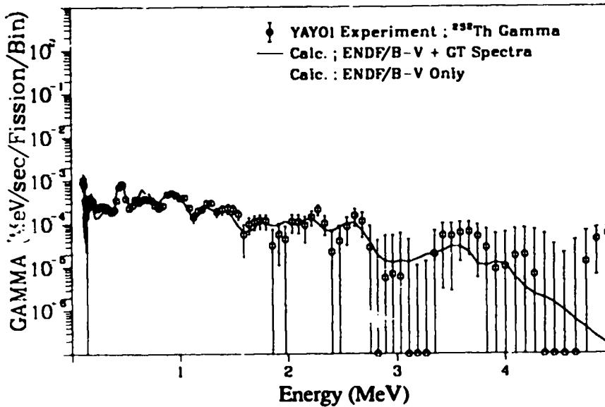
Fig. 345. Gamma spectrum after  $^{232}\text{Th}$  fast neutron fission
