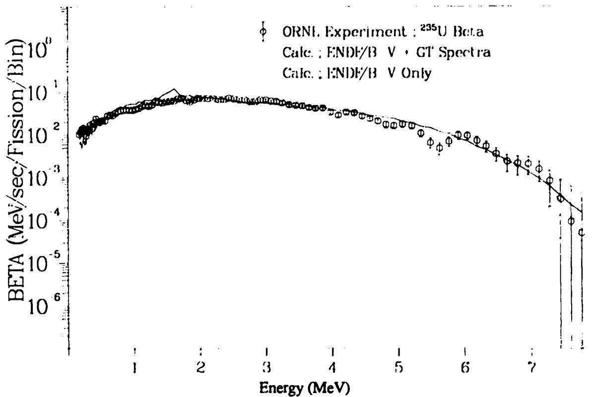
Fig. B-2. Beta-ray spectrum after  $^{235}\text{U}$  thermal neutron fission ( $T_{\text{irrad.}} = 1.0 \text{ sec}$ ,  $T_{\text{cool.}} = 2.2 \text{ sec}$ ) (to 8 MeV).
