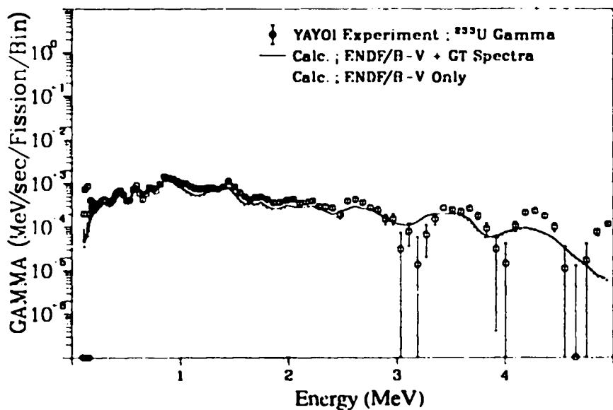
Fig. 170. Gamma spectrum after  $^{233}\text{U}$  fast neutron fission
