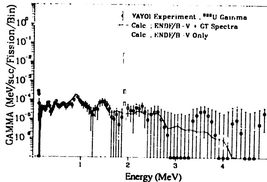
Fig. 262. Gamma spectrum after  $^{238}\text{U}$  fast neutron fission
