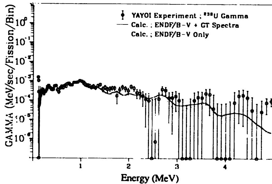
Fig. 252. Gamma spectrum after  $^{238}\text{U}$  fast neutron fission
