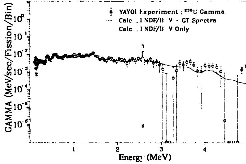
Fig. 191. Gamma spectrum after  $^{235}\text{U}$  fast neutron fission
