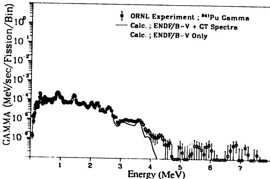
Fig. 142. Gamma spectrum after  $^{241}\text{Pu}$  thermal fission
