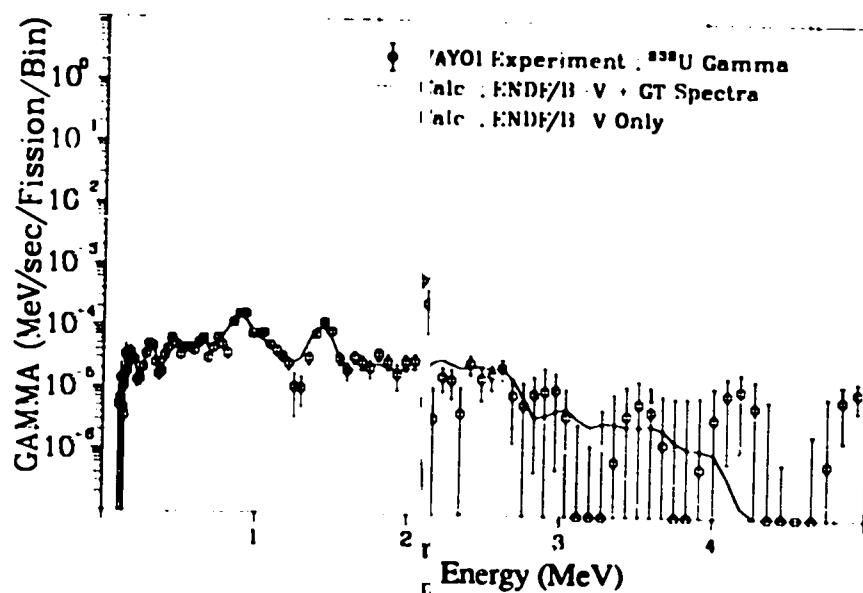
Fig. 212. Gamma spectrum after  $^{235}\text{U}$  fast neutron fission
