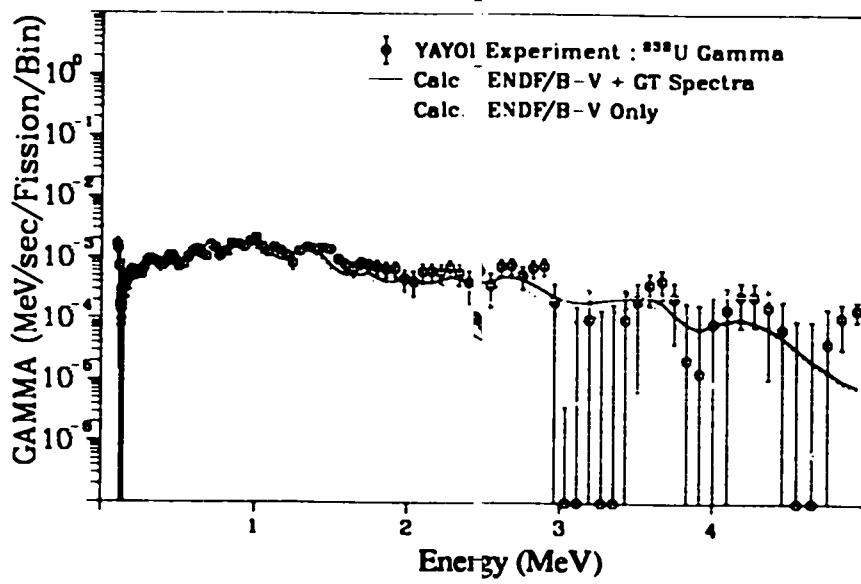
Fig. 249. Gamma spectrum after  $^{238}\text{U}$  fast neutron fission
