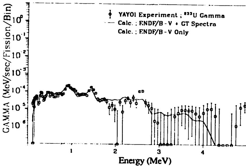
Fig. 166. Gamma spectrum after  $^{233}\text{U}$  fast neutron fission
