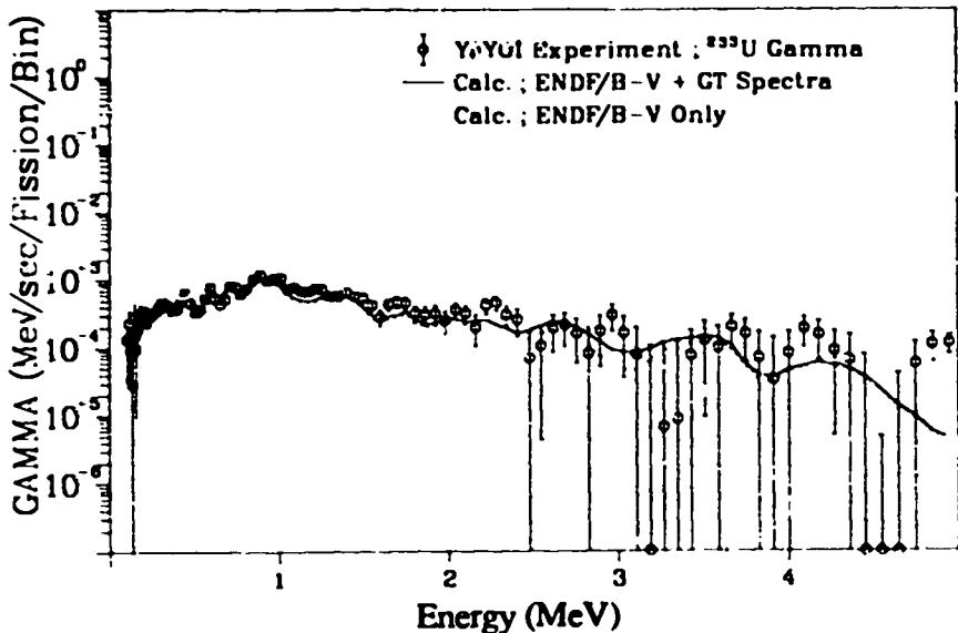
Fig. 201. Gamma spectrum after  $^{235}\text{U}$  fast neutron fission
