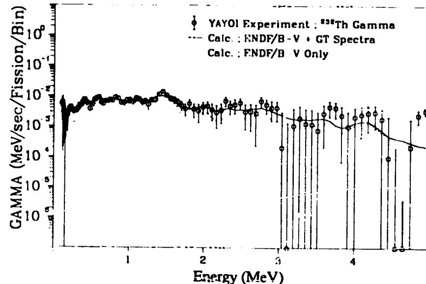
Fig. 332. Gamma spectrum after  $^{232}\text{Th}$  fast neutron fission
