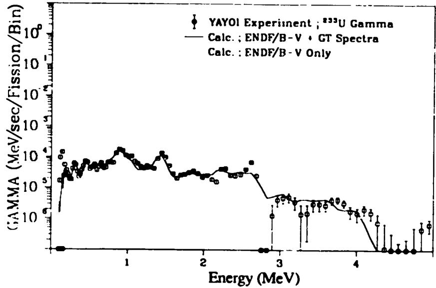
Fig. 177. Gamma spectrum after  $^{233}\text{U}$  fast neutron fission
