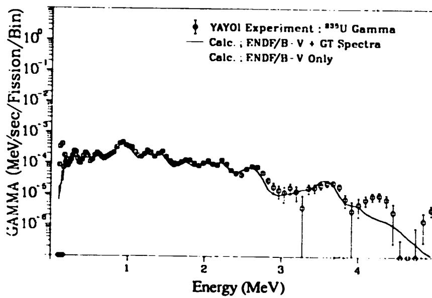
Fig. 222. Gamma spectrum after  $^{235}\text{U}$  fast neutron fission
