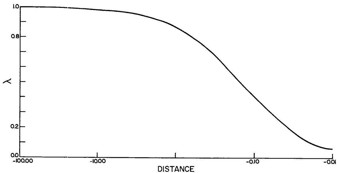
Fig. 11. Reaction extent \lambda vs distance.
