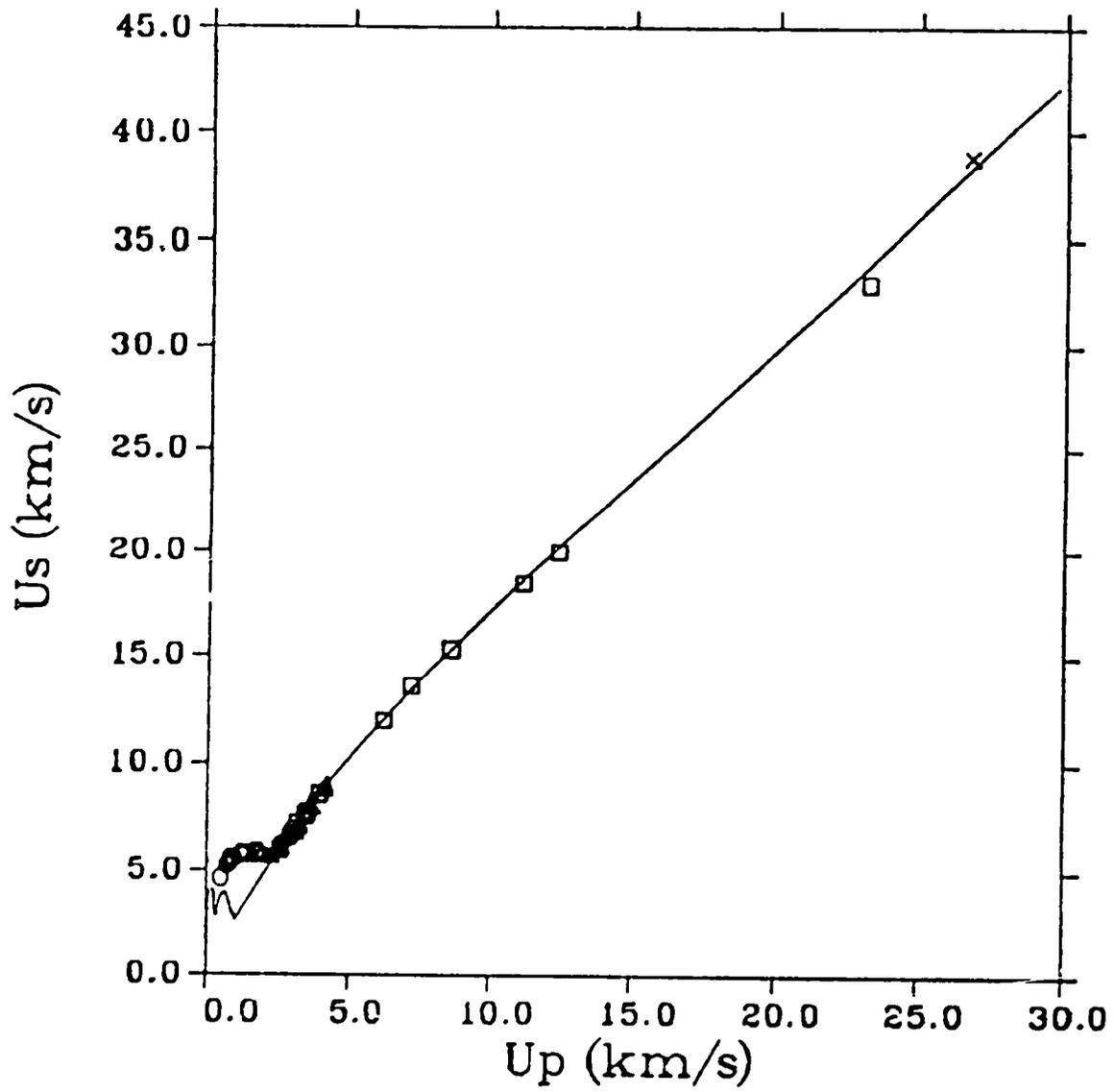
Fig. 2. Theoretical  $u_s$  vs  $u_p$  curve (line) compared with experiment (circles - Ref. 14, triangles - Ref. 15, squares - Ref. 16, crosses - Ref. 17). See Fig. 3 for a close up view of the small  $u_p$  region.
