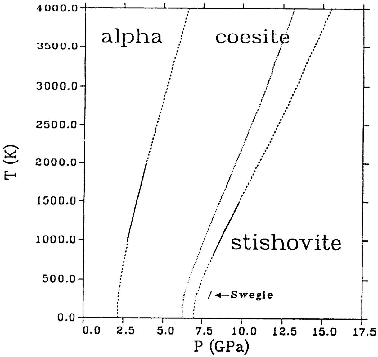
Fig. 1. The theoretical phase diagram for  $SiO_2$  (dashed lines) compared with the experimental alpha  $\rightarrow$  coesite (Ref. 10) and coesite  $\rightarrow$  stishovite (Ref. 11) boundaries (solid lines). Also shown are the hypothetical alpha  $\rightarrow$  stishovite boundary obtained here (dotted line) and that used by Swegle (Ref. 1).
