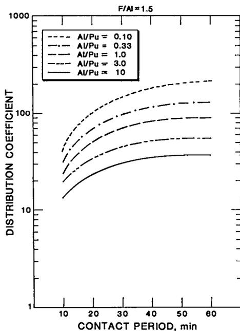
Fig. 7. Sorption of Pu(IV) on Lewatit MP-500-FK anion exchange resin from 7 M nitric acid that contains varying ratios of aluminum to plutonium for  $F/AI = 1.5$ , as a function of dynamic contact time.
