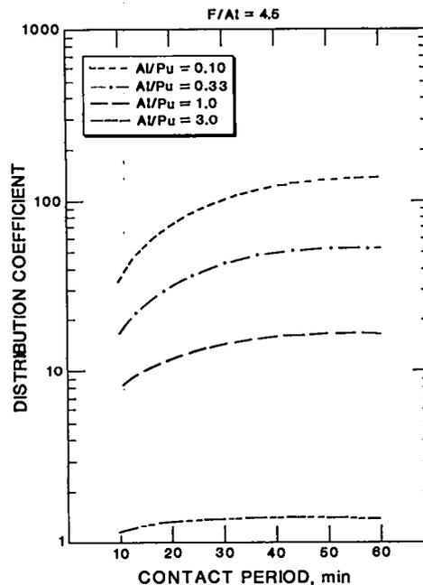
Fig. 9. Sorption of Pu(IV) on Lewatit MP-500-FK anion exchange resin from 7 M nitric acid that contains varying ratios of aluminum to plutonium for  $F/AI = 4.5$ , as a function of dynamic contact time.
