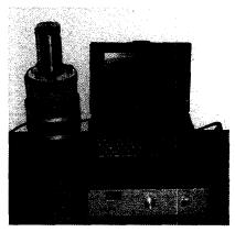
used in Idaho national Engineering and Environmental Laboratory's PINS system. This provides a high-performance system that is also radiologically safe and environmentally clean. The method is highly penetrating, illuminating 1-meter depths in common objects. The tool will be useful in explosives detection, humanitarian demining, anti-smuggling of contraband, and oil- and gas-well analyses.
