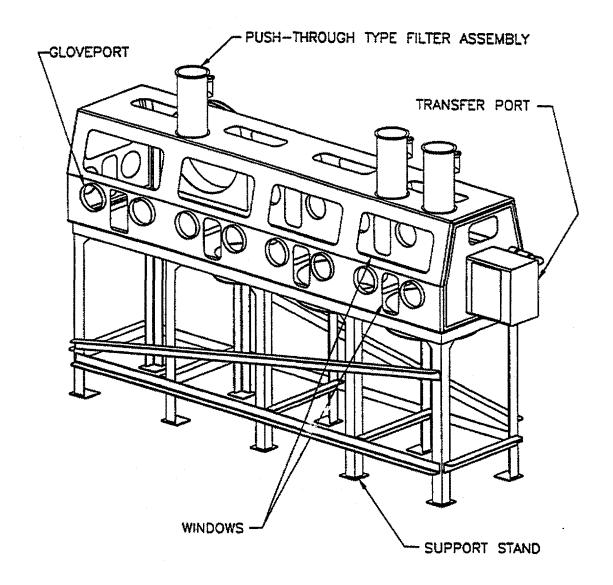
Figure 1. Sketch of a typical glovebox (from American Glovebox Society, report AGS-G001-1998).
