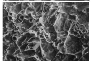
Figure 1: These optical micrographs show crystallographic or faceted pitting of 304 SS following a one-week immersion in 4.1 M nitric acid plus 1 M sodium chloride. Microscopy was one of a variety of approaches within the overall research program to evaluate the influence of environmental and material effects on the corrosion behavior of stainless steel exposed to simulated waste-processing environments.
