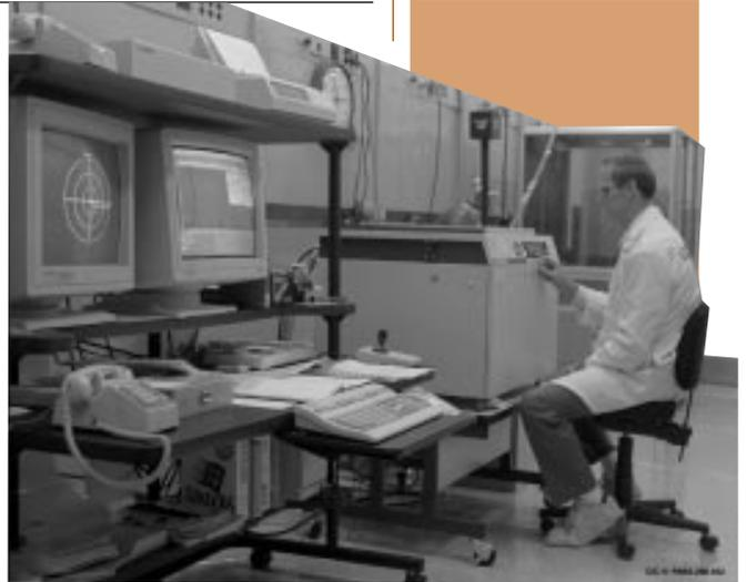
**Joel Dahlby, CST-8, operates an x-ray microfluorescence instrument, an innovative use of XRF to excite a specific location on a specimen. The technique can be used to perform spatially resolved elemental analysis for concentrations of 10 ppm to weight percent levels.**
