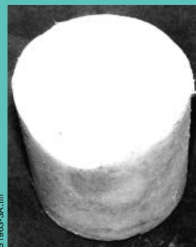
Figure 1. Top photo: a 1.5 kg (approx.) example of contaminated salt residue. Below left: After treatment using the high-temperature vacuum distillation method, the condensed salt distillate can be discarded as low-level waste. Below right: The plutonium contaminant, now in the form of a concentrated plutonium oxide, will be stored as special nuclear material.
