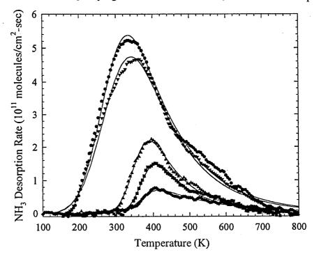
Figure 2. The low-coverage NH<sub>3</sub> TPD spectra (symbols) and the fits to the model (solid lines) for different values of the initial coverages  $\theta_{0.}$  ( $\theta_0 = 0.003$ , 0.006, 0.024, and 0.026 ML, from bottom to top.)
