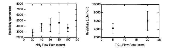
Figure 18. Four-point probe measurements of film resistivity as a function of ammonia (left) and titanium tetrachloride (right) flow rate.
