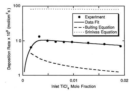
Figure 6. Optimized fit of deposition data from Sandia/MRC rotating disk reactor.
