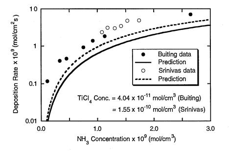
**Figure 9.** Predicted NH<sub>3</sub> dependence of the TiN deposition rate vs. deposition rates (adjusted to 903 K) reported by Buiting et al. and Srinivas et al.
