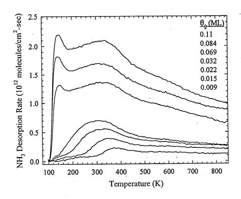
Figure 1. Temperature-programmed desorption spectra of increasing coverages of NH<sub>3</sub> from TiN. Curves for  $\theta_0$  varying from 0.009 to 0.11 ML, from bottom to top.
