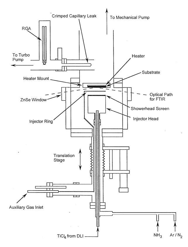
Figure 11. Cross-sectional view of the stagnation-flow reactor.
