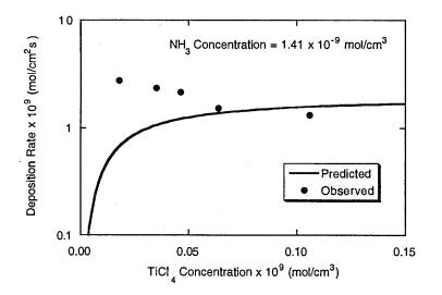
Figure 7. Predicted TiCl<sub>4</sub> dependence of the TiN deposition rate vs. observed deposition rates (adjusted to 903 K) reported by Buiting et al.
