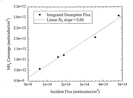
Figure 3. Surface coverage of NH<sub>3</sub> vs incident flux. The slope of the line gives the sticking probability.
