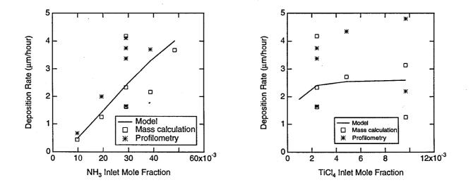
Figure 19. Dependence of the TiN deposition rate on inlet reactant NH<sub>3</sub> (left) and TiCl<sub>4</sub> (right) mole fractions. Deposition conditions are as described in the text.
