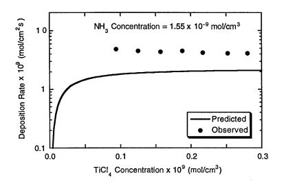
**Figure 8.** Predicted TiCl<sub>4</sub> dependence of the TiN deposition rate vs. observed deposition rates (adjusted to 903 K) reported by Srinivas et al.
