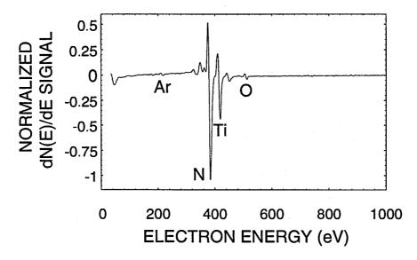
Figure 15. Auger spectrum of the as-received TiN film (top) and after sputtering for one hour with 5 KeV argon ions (bottom).
