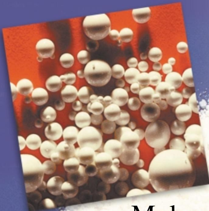
Beads of anion-exchange resin are used in the nitric acid plutonium recovery process. The background shows a powder of Reillex™ 402 polymer, which was modified to produce new, highly sorbtive anion-exchange resins.
