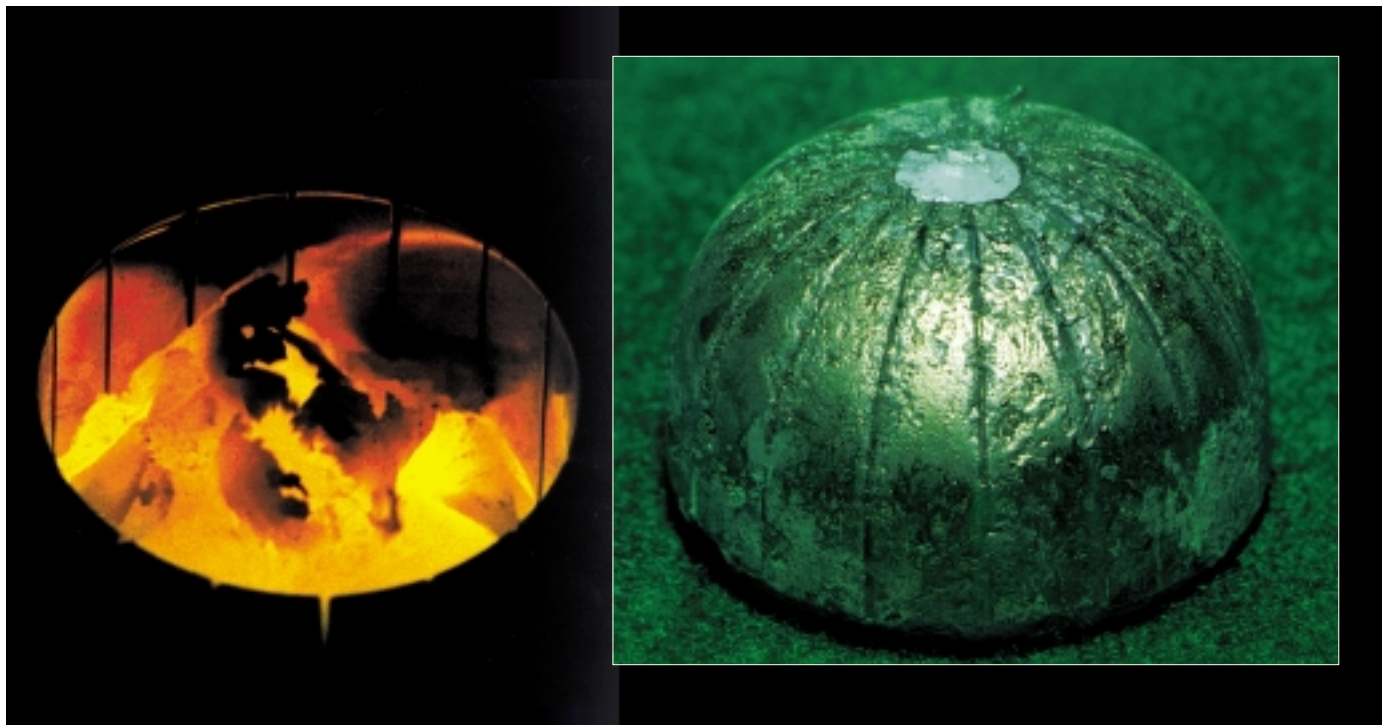
Figure 4. Vacuum Distillation of Plutonium Metal
