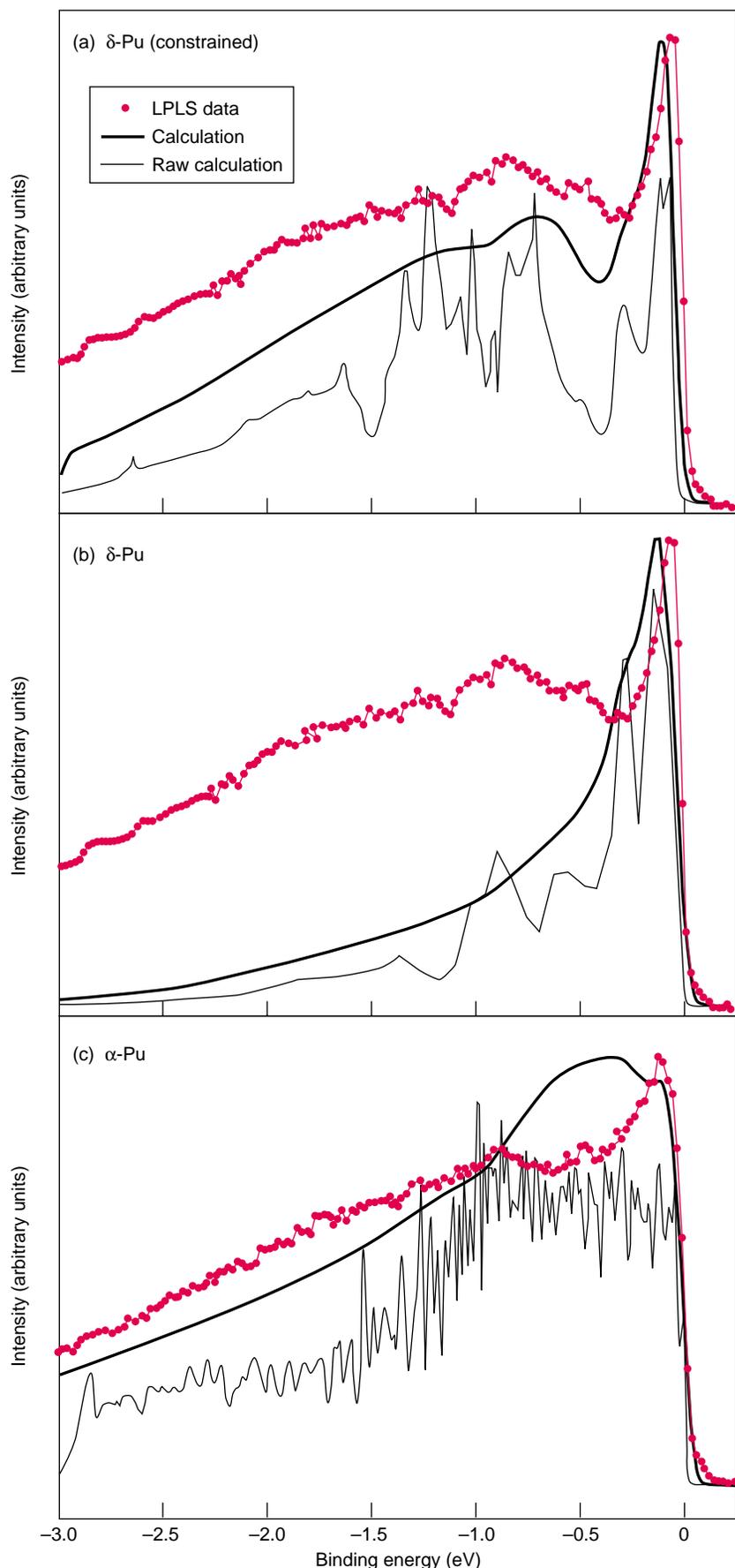
of states is found to be contained in a narrow region within 0.5 eV of the Fermi energy (similar to uranium results). This result is clearly at odds with experiment and reinforces the notion that at least some of the 5f electrons are localized.
