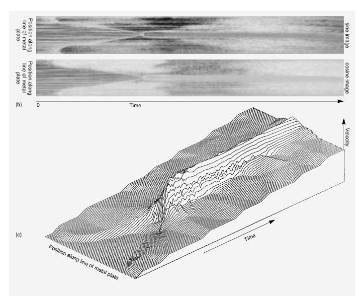
camera rapidly sweeps the images across a charge-coupled device that digitizes them into a microcomputer. Later, we subtract one image of each polarization from its negative to double the signal and cancel optical noise. Analysis of the images yields the velocity histories of many points in the line as a continuous function of time.
