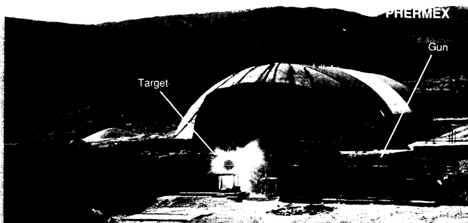
Fig. 2. A flash x-ray machine (in the building behind the target) is currently being used to produce high-resolution radiographs (see Fig. 4) of the ballistic interaction of ceramic targets with long-rod penetrators (fired from the gun at the right).
