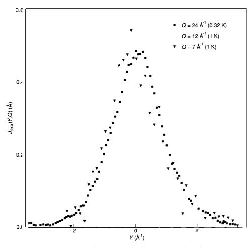
chopper spectrometer optimized for momentum-distribution studies. The spectrometer, known as Phoenix, was built at the Intense Pulsed Neutron Source at Argonne National Laboratory. Phoenix has provided data at Q values up to 24 Å $^{-1}$ . The pulsed-source experiments thus more closely approach conditions at which the impulse approximation might be valid. They also permit much greater control of the instrumental resolution function than do reactor experiments.
