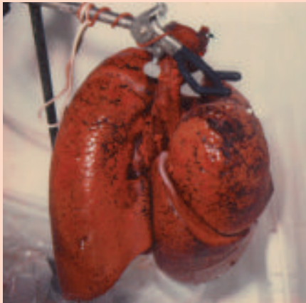
Lungs from an occupationally exposed worker inflated with dry nitrogen to approximately normal size found in the human chest. The ratio of plutonium to americium was measured in the Los Alamos lung counter and compared with measurements made before death.
