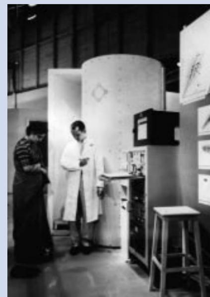
In 1958, the human counter was demonstrated at the Atoms for Peace Conference held in Geneva. Built especially for this conference, the vertical counter was open on one side to allow a person to step in for measurement of internal radioactivity. The middle picture shows a conference participant getting ready to enter the detector under Newton Hayes’ supervision.
