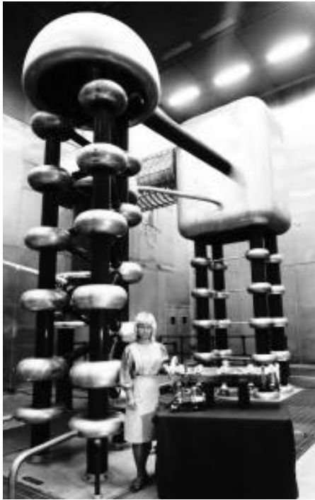
An RFQ Cavity. The accelerator is shown here in front of the accelerator it may someday replace—the LAMPF Cockcroft-Walton.
