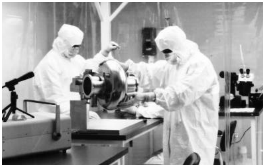
The Clean Room at Accelerator Technology Division. Superconducting accelerator cavities of niobium are fabricated under conditions of extreme cleanliness.
