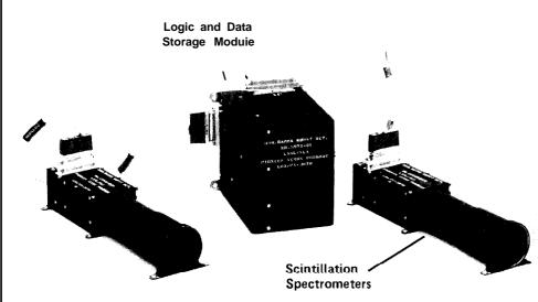
The gamma-ray detection system aboard the Pioneer Venus Orbiter spacecraft.
