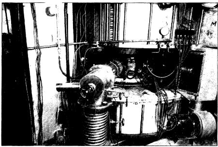
The cyclotron commandeered for use at Los Alamos belonged to Harvard University and had been built there during the 1930s. It produced 7-MeV protons and 11-MeV deuterons with a maximum beam current of 100 microampere. The two largest pieces of its magnet each weighed 18 tons, and the magnet's total weight was 70 tons. In preparation for
