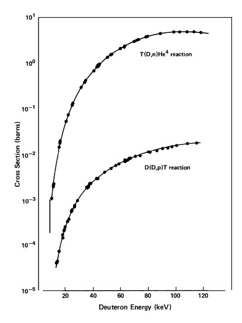
Definitive measurements were made at Los Alamos in the early 1950s of the cross sections for two fusion reactions that might form the basis of a thermonuclear weapon. From W. R. Arnold, J. A. Phillips, G.A. Sawyer, E. J. Stovall, Jr., and J. L. Tuck, Los Alamos Scientific Laboratory reports LA-1479 and LA-1480 (January 1953).
