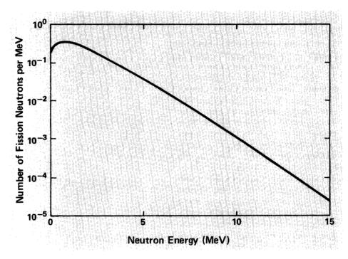
Accelerators were brought to Los Alamos to provide neutrons with energies similar to those of the majority of neutrons produced by fission of uranium-235 or plutonium-239. Shown here is the spectrum of neutrons emerging from the fission of uranium-235; the fission neutron spectrum of plutonium-239 is similar.
