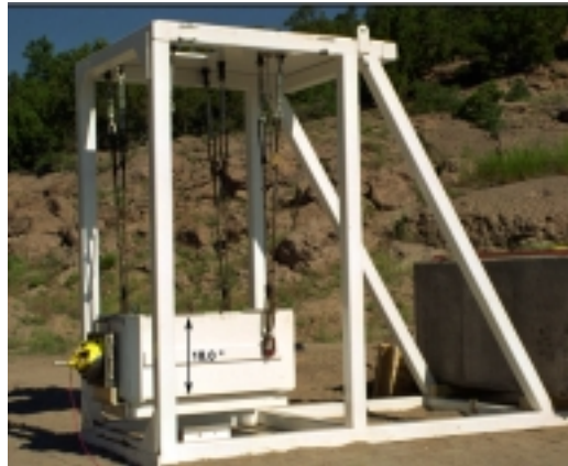
Figure 5. Ballistic pendulum with a PBX 9501 calibration target attached.
