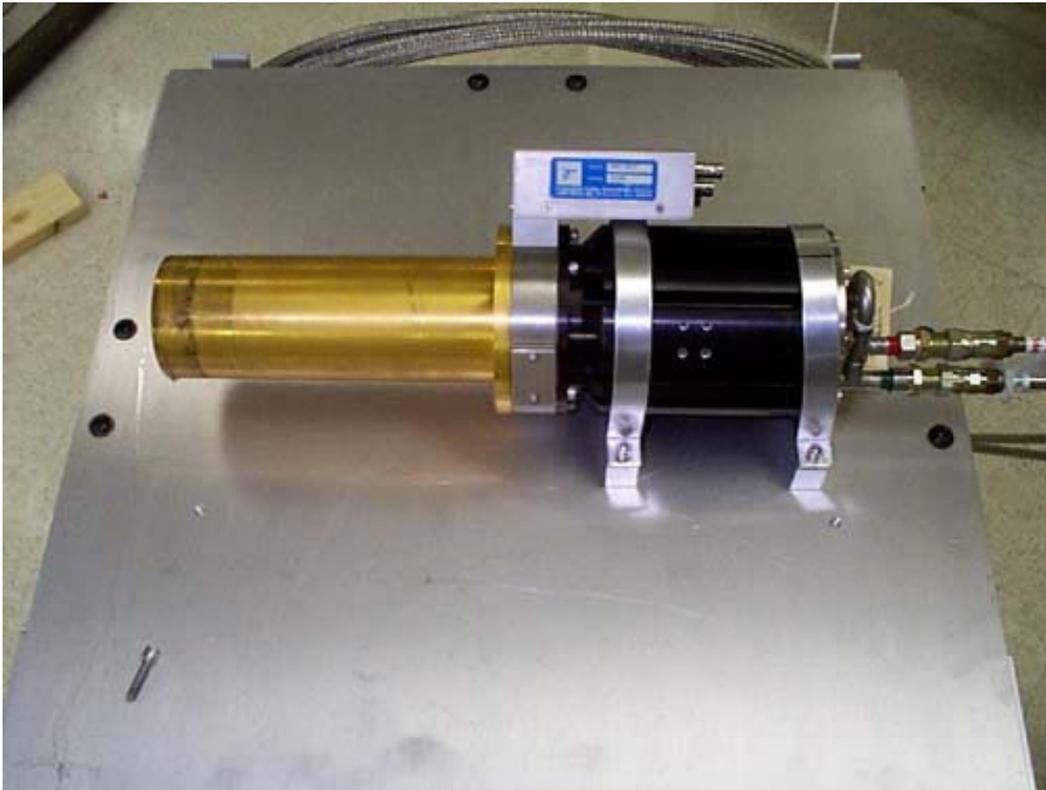
Figure 46. The detector head is supported by two “saddles” on the top shelf of the frame. The U-clamps attached to the saddles hold the detector in place.
