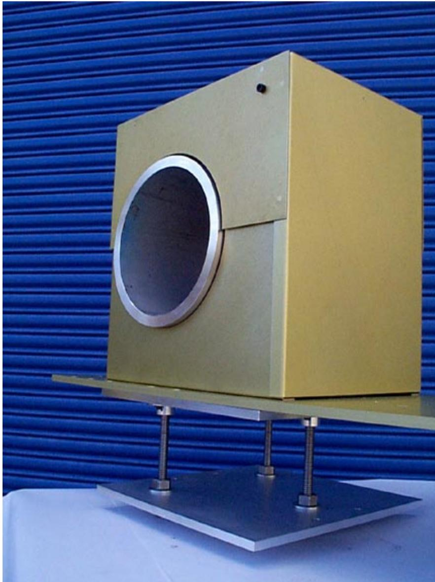
Figure 57. The 8-in. (20.32-cm) collimator and TIE are attached to a plate. Three threaded rods, used for height adjustment, attach this plate to a second plate that is subsequently attached to a frame (not shown in the figure) made of 80/20 aluminum extruded stock. This 80/20 frame sits directly on the floor beneath the header pipe.
