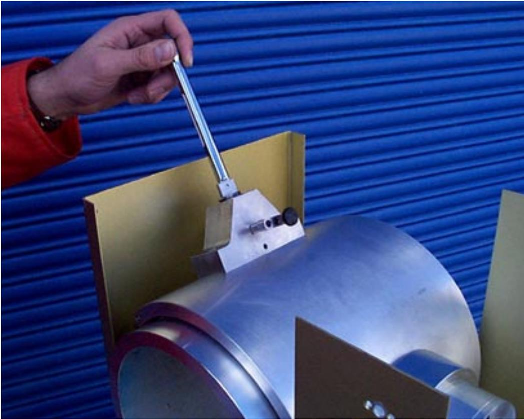
Figure 62. A “socket driver” is used to place the XRF source plug in the source housing. Tighten finger tight. Seal the XRF source plug using the eyelet on the source housing. This will keep the source plug from coming loose because of vibrations of the header pipe.
