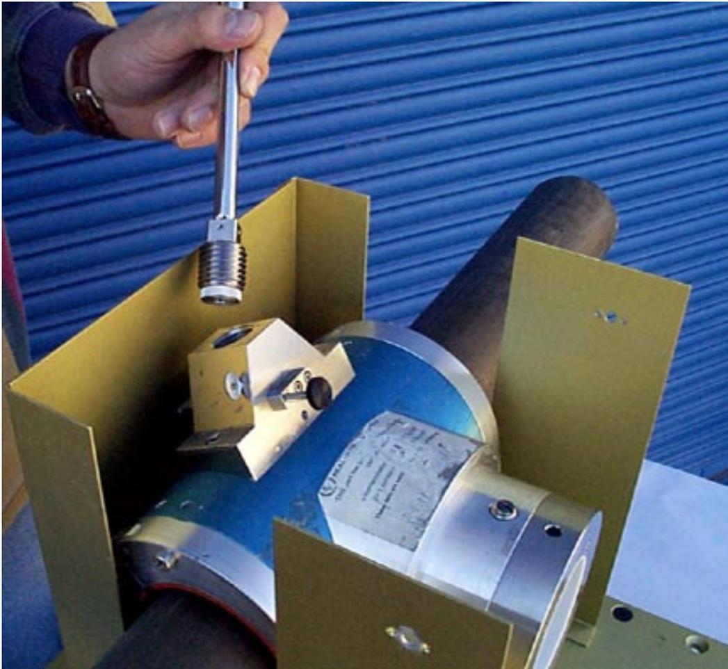
Figure 53. The XRF source is located in the end of the threaded tungsten source plug, behind the aluminum retainer cap.
