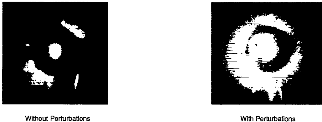
Fig. 11. X-ray images of ablative cylindrical implosions with and without imposed perturbations.
