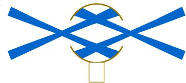
By changing to a spherical geometry and pointing the beams so that they cross at the laser entrance hole, the angle of incidence decreases to 22.5° from perpendicular.
