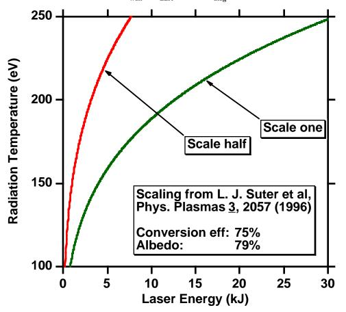
hole, and diagnostic hole areas, respectively. In the figure below, the comparisons are calculated using this formula and the values for conversion efficiency ( $\eta$ =0.75) and albedo ( $\alpha$ =0.79) used in reference [Suter 96a] for Nova hohlraums.
