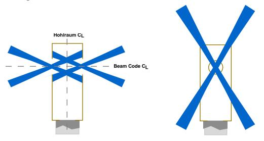
Depending on the details of the design, these hohlraums might have reduced illumination uniformity on the experimental package. In addition, for the design shown above, the laser entrance hole size is limited by the size of the circle of beam spots formed around it.
