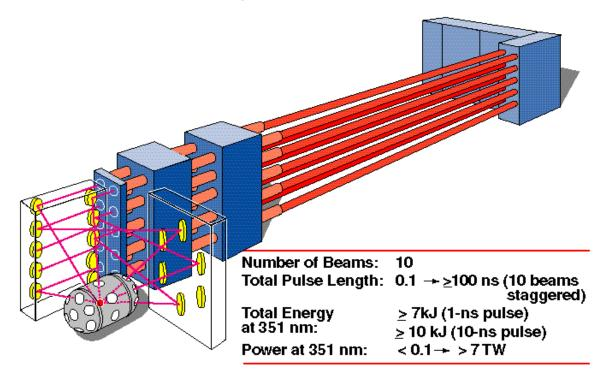
end, with a half angle of 22.5°, and that there will be eight evenly spaced beam ports around the equator. It is further assumed that no more than 10 of these beams will be available at any given time to drive a hohlraum.
