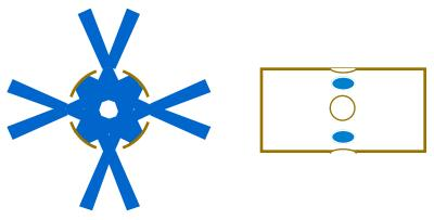
Alternatively, if the beams are not directly on the midplane of the target chamber, or if the LEHs are staggered so that two are closer to each end, then a larger LEH can be used, or greater distance from the beam spots to the LEHs could be realized.
