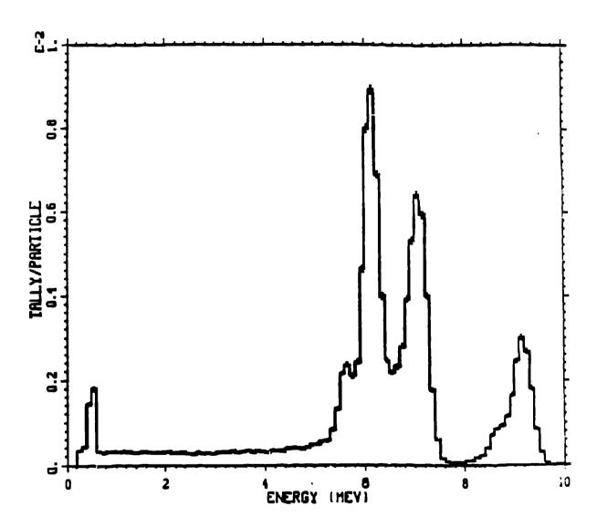
MCNP simulation of the 3" x 3" BGO monitor detector with a multiple gamma-ray source from the composite target.
