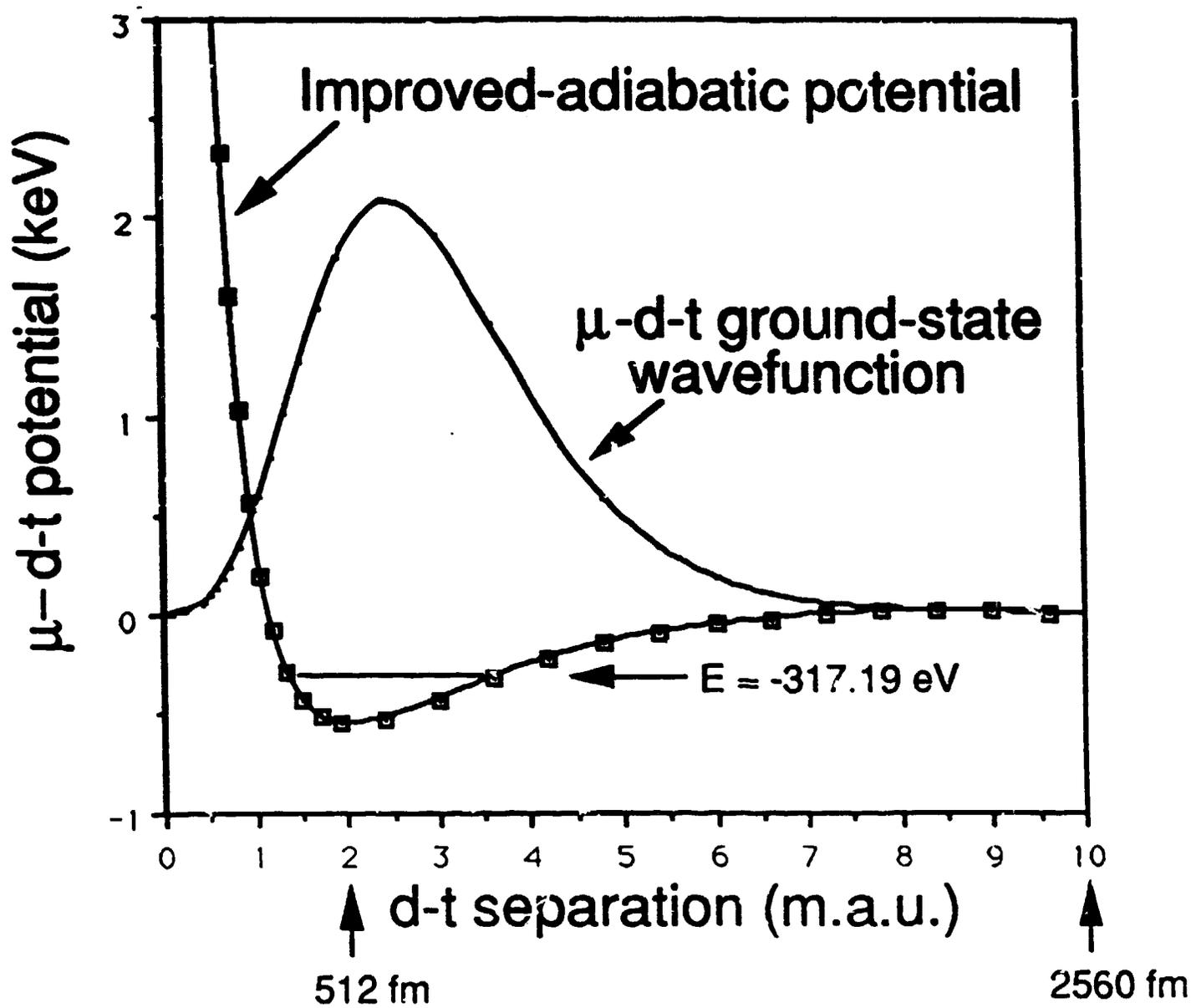
Fig. 5. Improved adiabatic  $d\mu$  potential (squares) and ground-state radial wavefunction (solid line) as functions of  $d$ - $t$  separation in muonic atomic units. The ground-state energy of the molecule is also shown relative to the mass of  $d+t\mu$ .
