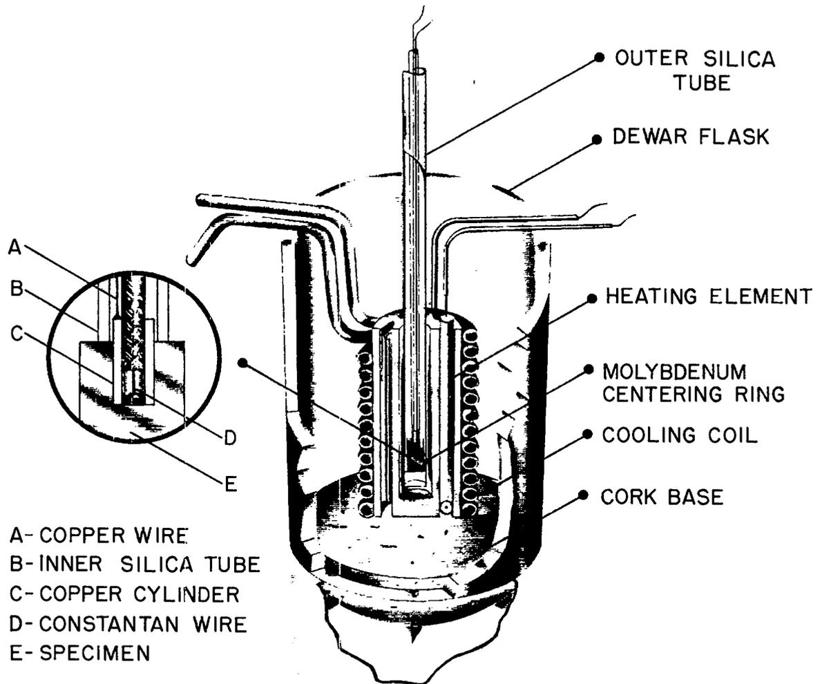
Figure 4. Location of dilatometer specimen.
