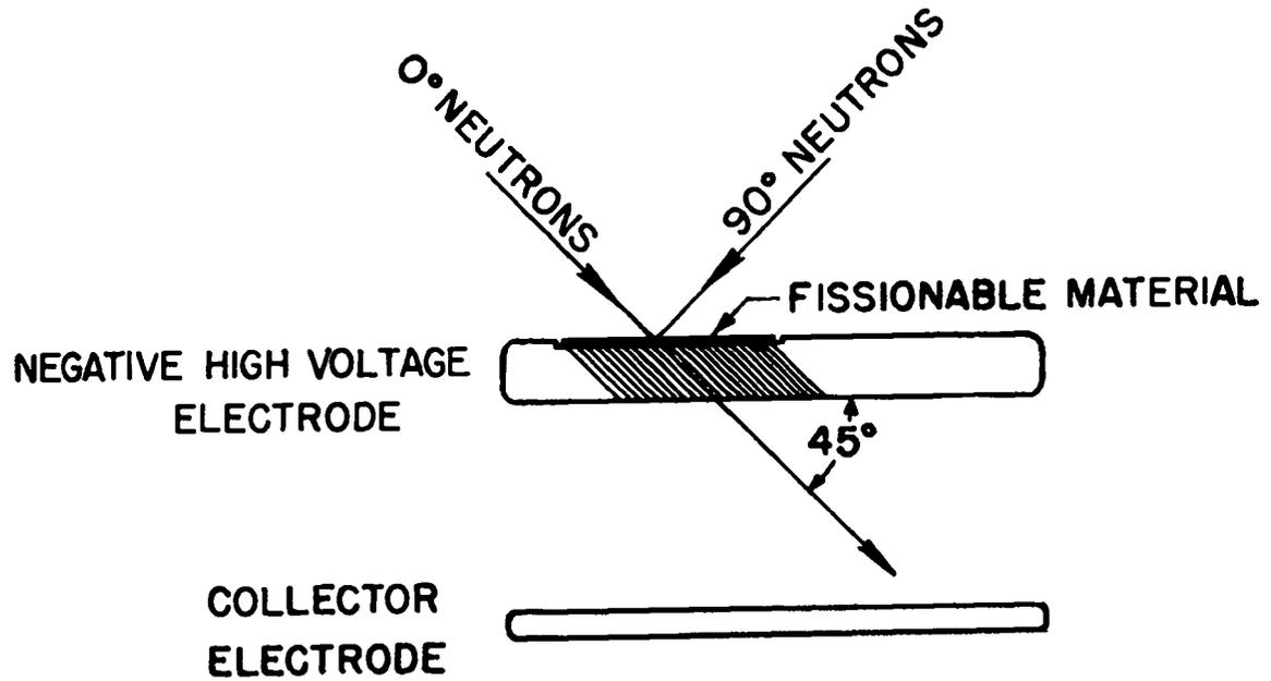
Fig. 2. Schematic representation of the fission chamber.
