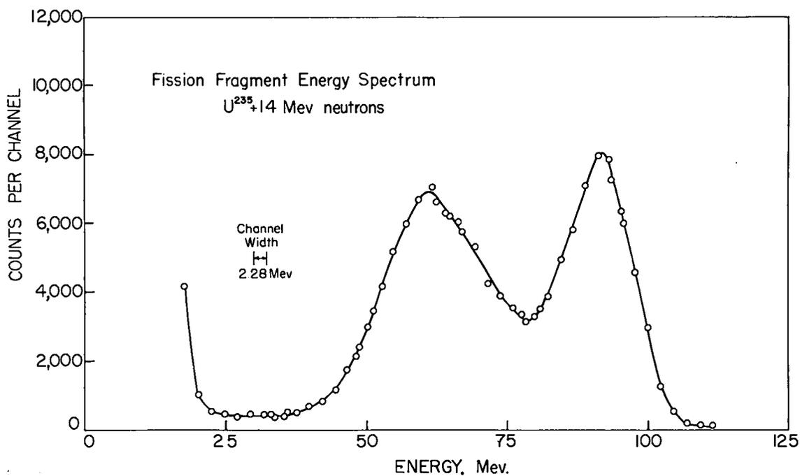
Fig. 6. Fission fragment energy spectra for thermal and 14-Mev neutrons.
