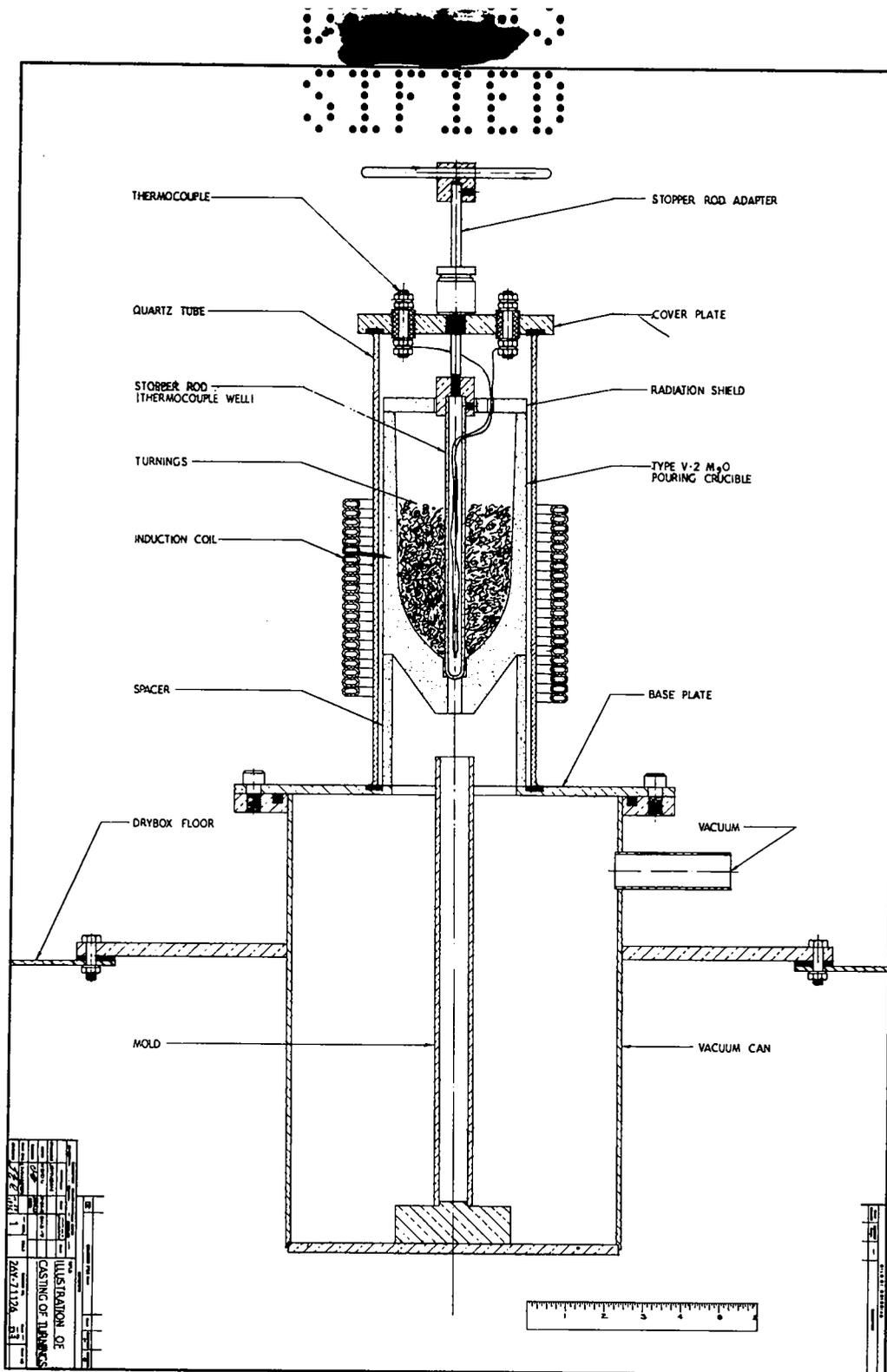
Fig. 3. Cross Section of Casting Unit.
