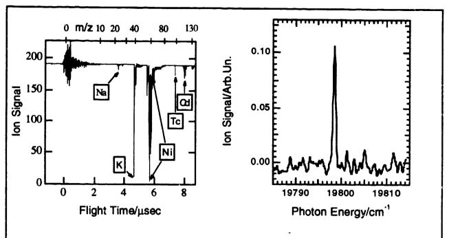
Figure 2a shows a mass spectrum resulting from resonant laser ablation of Tc from a Nickel sample, using the  $e^6S_{5/2} \leftarrow a^6S_{5/2}$  two photon transition shown in 2b.
