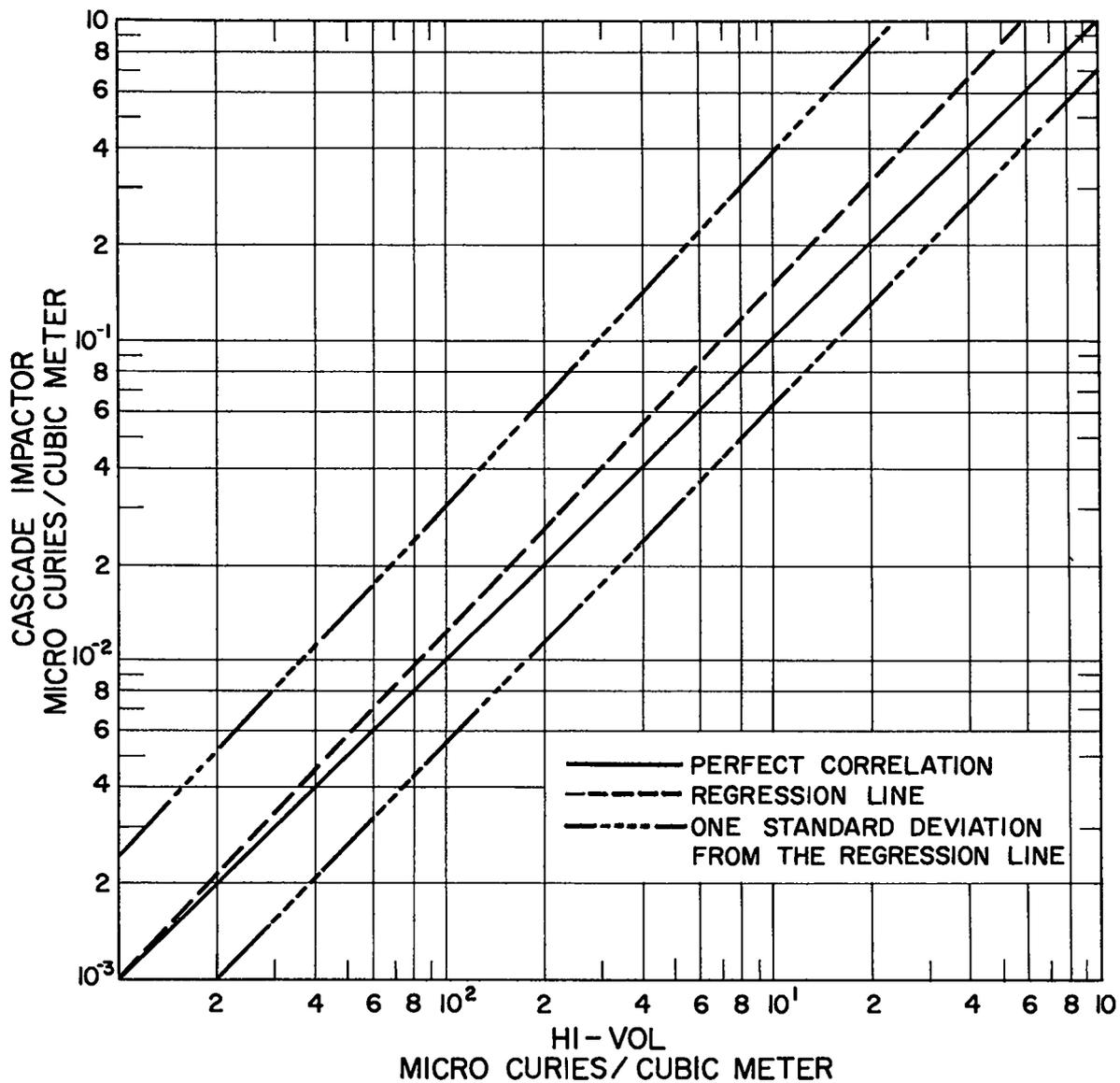
Fig. 26. Air concentration. Comparison of the High-Volume sampler and the cascade impactor.
