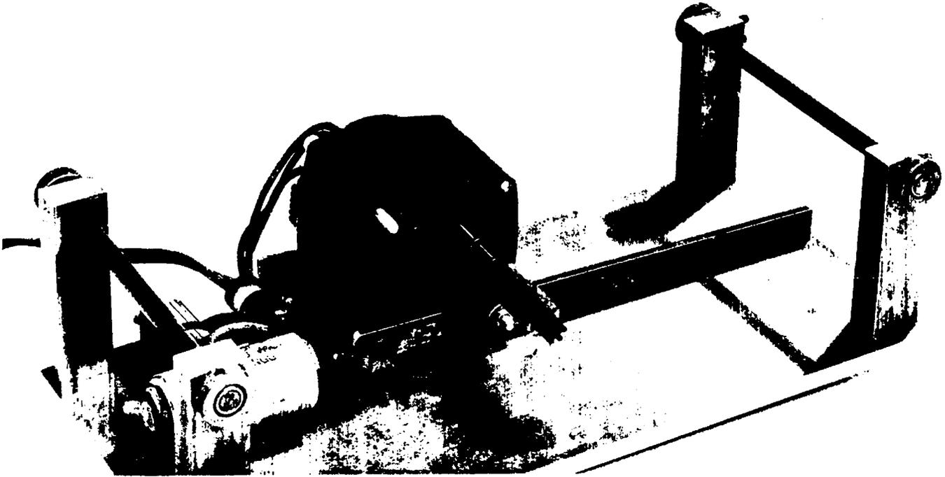
Fig. 3. Motor-driven carriage
