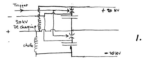
The circuit of Fig. 1 allows one to do this in a nice way without requiring or producing more than 20 kV with respect to ground using the present Sherwood condensers. In effect, the condensers are charged in parallel, but discharge in series + and - with respect to ground.
