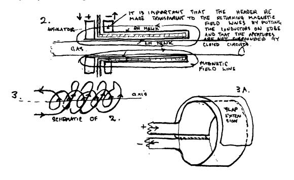
This will effectively give electromagnetic symmetry, and also makes it possible if needed, to slip the HE over the coil at the last minute.
