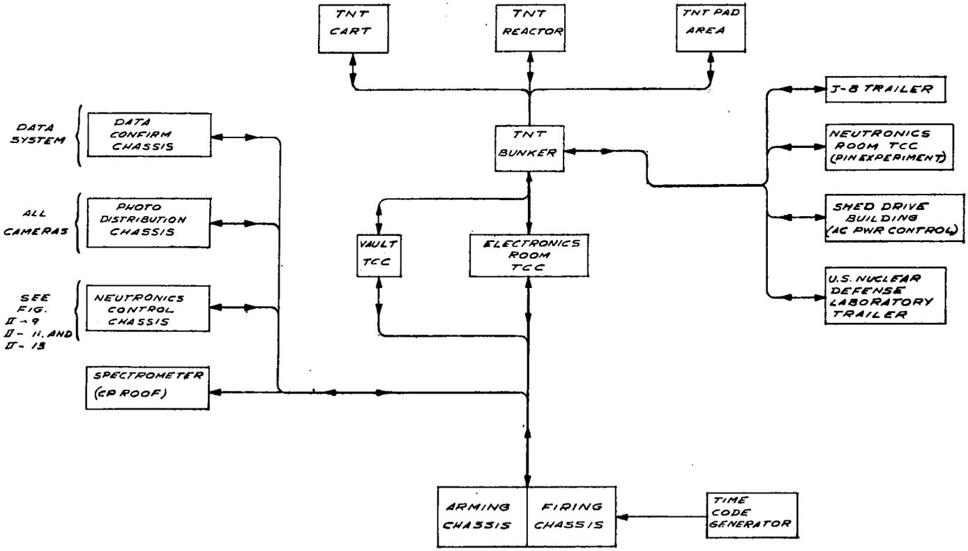
Figure 2-6. Control System Signal Flow Diagram
