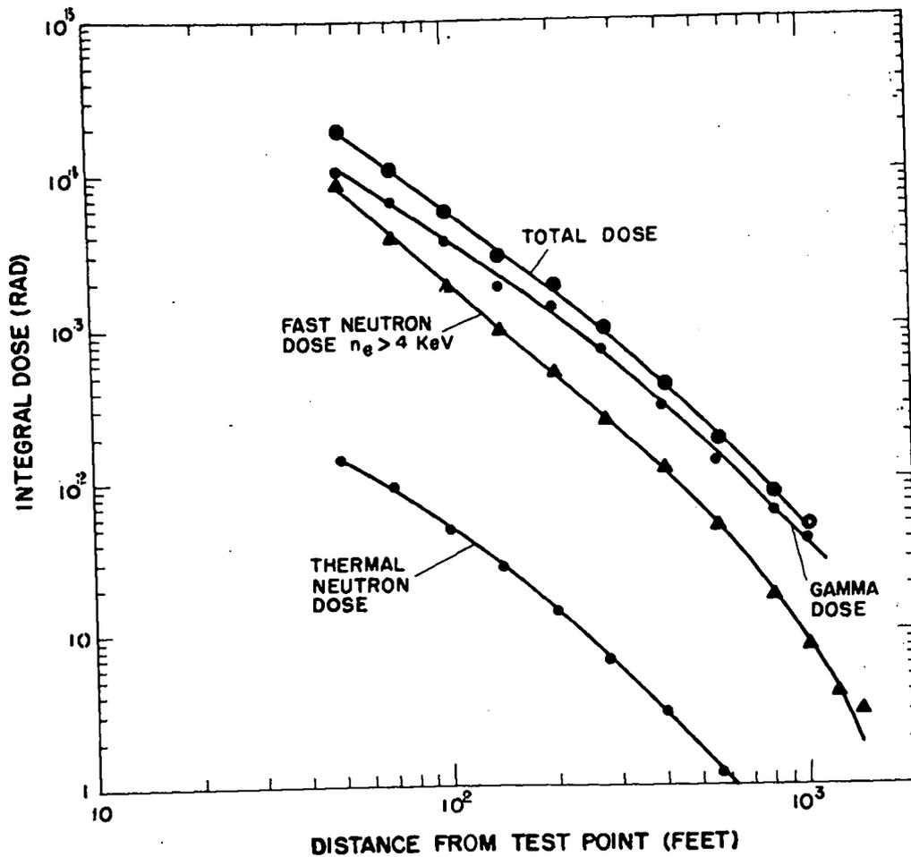
Figure 4-12. Integral Doses as a Function of Distance
