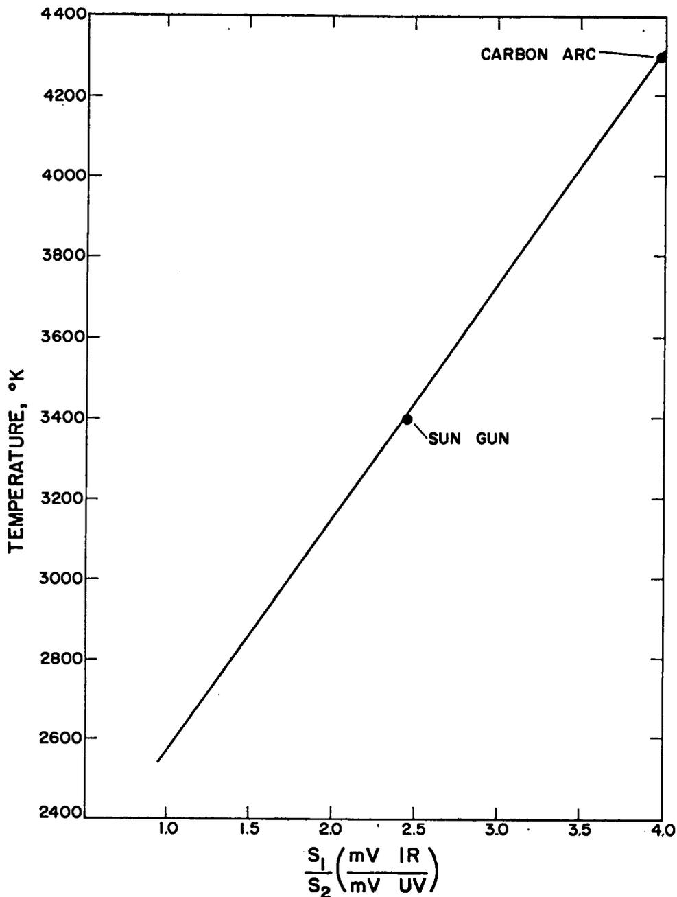
Figure 2-15. Temperature Calibration Curve, Lead Sulfide Detectors
