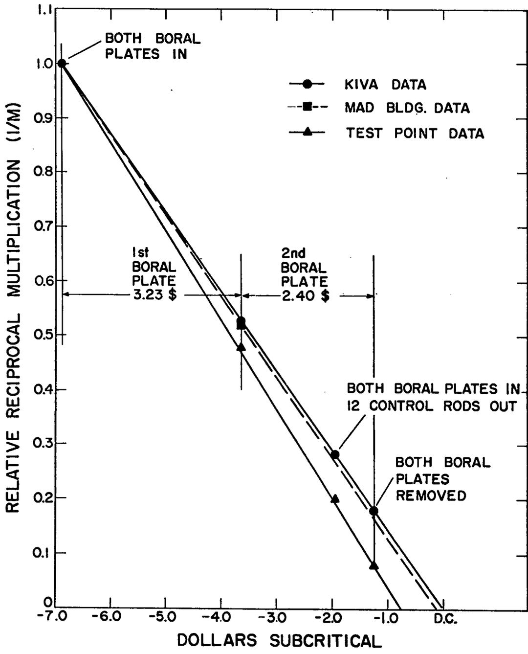
Figure 3-10. Reactivity of TNP for Various Poisoned Configurations
