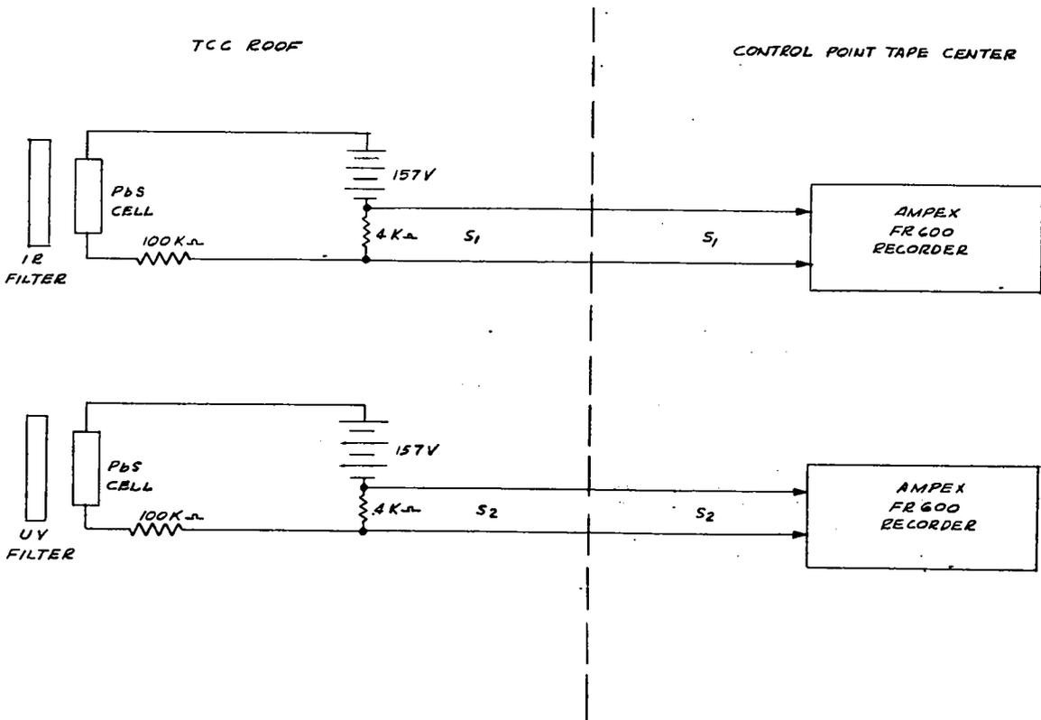
Figure 2-14. Signal Flow Diagram Fireball Temperature Estimate
