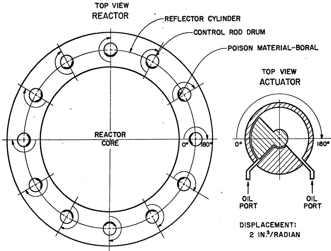
Figure 3-6. Twelve Control Rod Drum Layout Schematic
