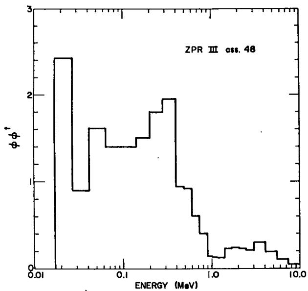
Fig. F-3. Reactivity weighing function  $\phi\phi^+$ ( $r = 0$ ) in ASSEMBLY 48.
