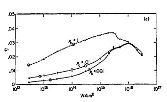
Fig. 1. Results of a numerical simulation parameter study of laser-driven implosion of solid spherical pellets. As a function of power, watts/cm² at the initial pellet surface, and critical density,  $\rho_{\text{C}}$ , the figures show a) peak values of  $\rho R$ , b) internal energy in the compressed pellet core at the time of peak  $\rho R$ , and c) efficiency,  $\eta$ , of transfer of absorbed laser energy into the core energy shown in b).
