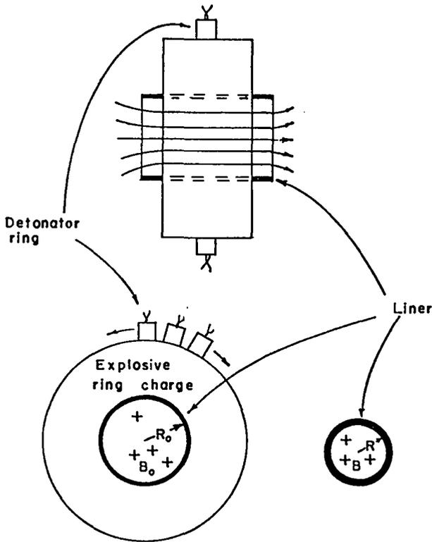
Fig. 6. Views of a cylindrical implosion system. The upper and lower left figures show the system before implosion. Cylindrical implosion is achieved by simultaneously initiating the row of high quality detonators mounted on the ring charge. The lower right figure shows a view of the liner at a later stage of the implosion.
