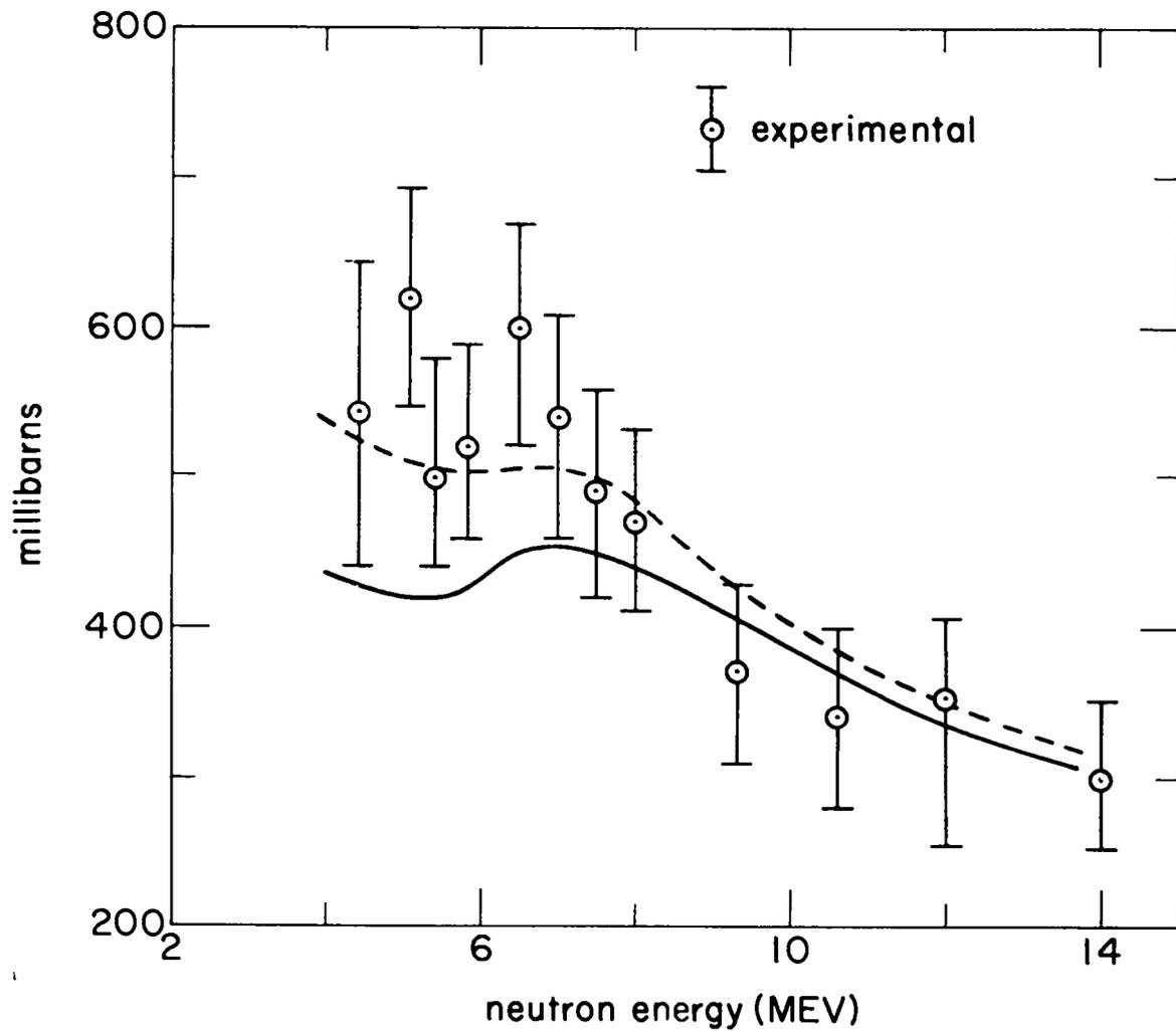
Fig. 1. Cross Section for  $n,d$  Reaction on  $\text{Li}^6$ . The solid line is the result of theory, including the compound nuclei and pickup. If an additional mechanism excites the 2.2 Mev state, the observed cross section for the latter leads to the dashed curve.
