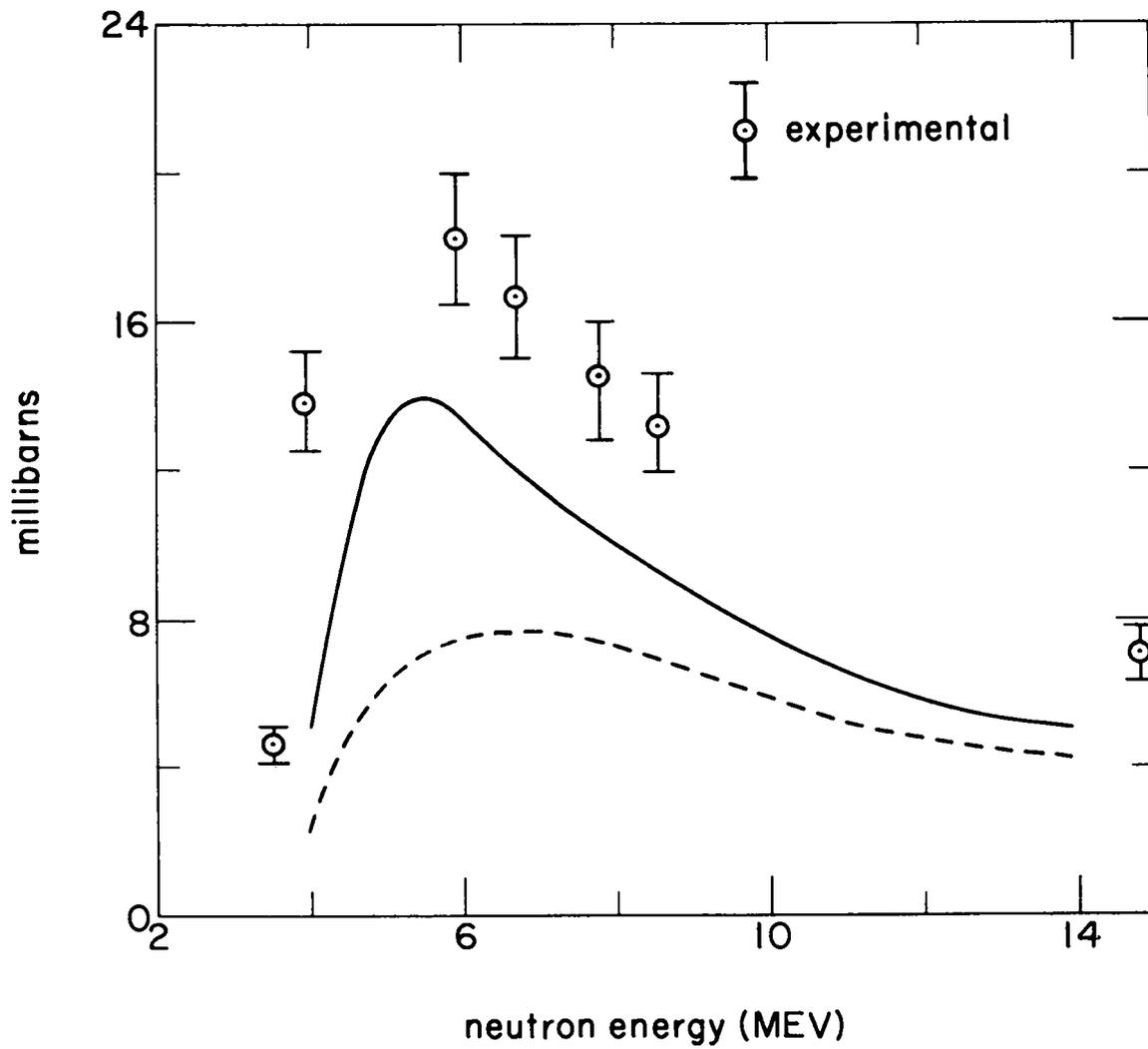
Fig. 5. Cross Section for n-p, He<sup>6</sup>
