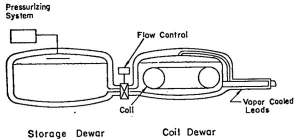
Fig. 6. Schematic of coil dewar and storage dewar.
