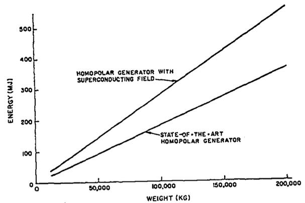
Fig. 2. Energy vs mass for homopolar generators.
