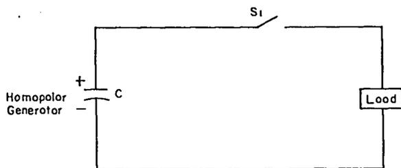
Fig. 4. Homopolar generator with direct load coupling.
