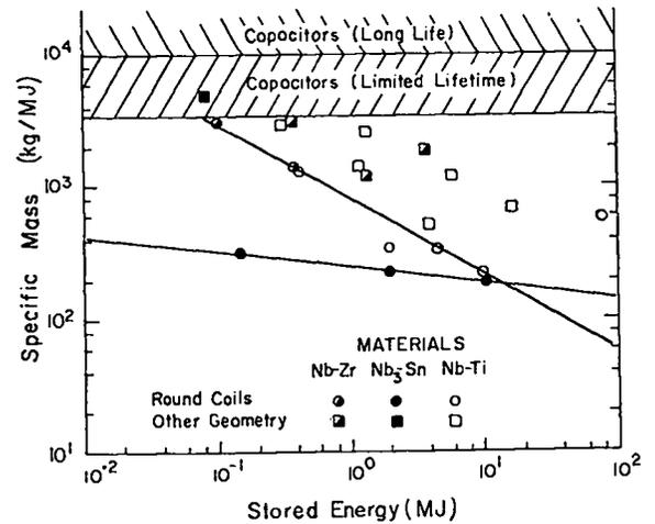
Fig. 5. Comparison of specific mass for capacitors (shaded) and current state-of-the-art superconducting coils (circles and squares).
