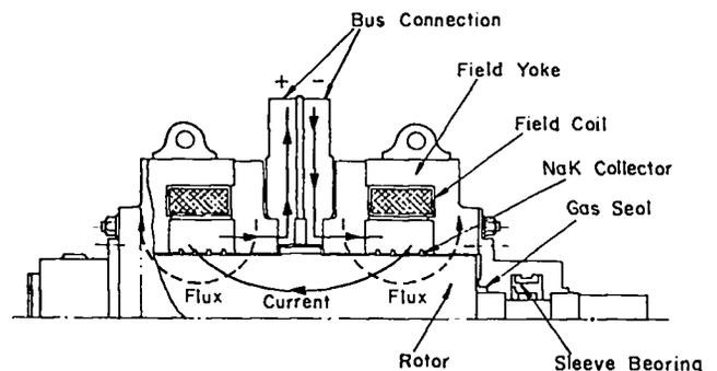
Fig. 1. Homopolar generator (from Ref. 1).
