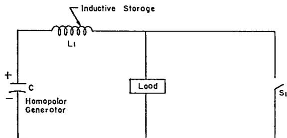
Fig. 3. Homopolar generator connected through a pulse-shaping inductive storage device to a load.
